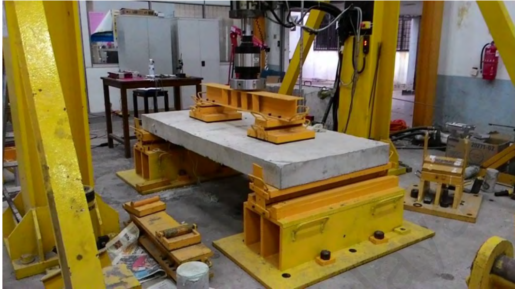
Figure 3.10: Test set-up and the support system with a hinged support at one end and a roller support at the other end
