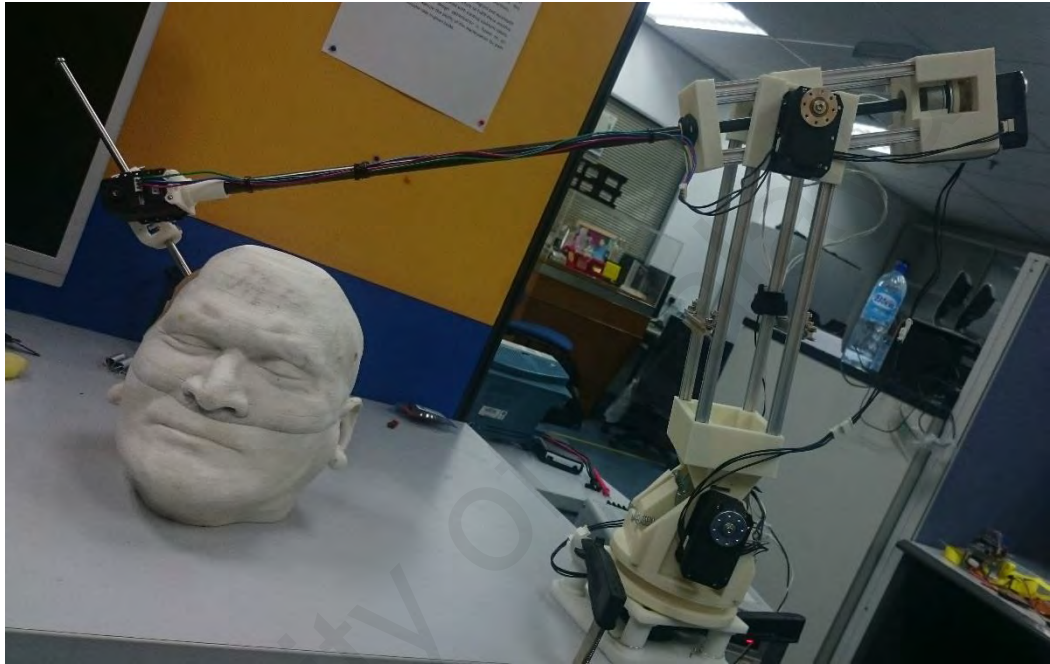
Figure 4.19 The second prototype uses electromagnetic brakes to keep the joints rigidly when it is needed. The joints were load balanced to put less pressure on the servo motors, at joint 2 two synchronized servo motors were used to handle the needed torque.
