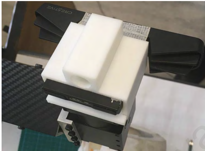
Figure 4.23 A bracket for the robot, designed to house a 3D camera and a cannula housing for needle placements.
