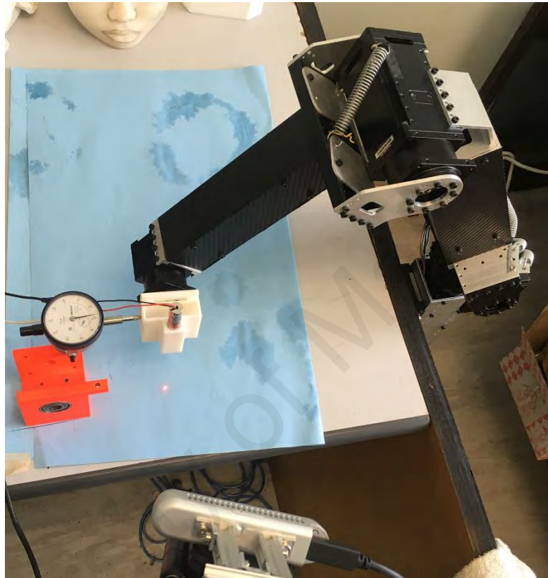
Figure 5.6 movement accuracy is tested using the dial indicator which has 1cm range. The robot was commanded to change the tool position along the indicator's plunger. The differences between the calculated forward kinematics and the indicator showed the error value. The camera and laser pointer are to measure the flex in the tip point.
