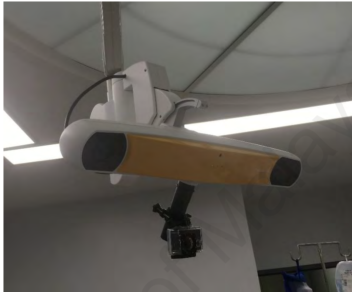
Figure 3.7 The image guidance optical tracker and the attached video camera.
