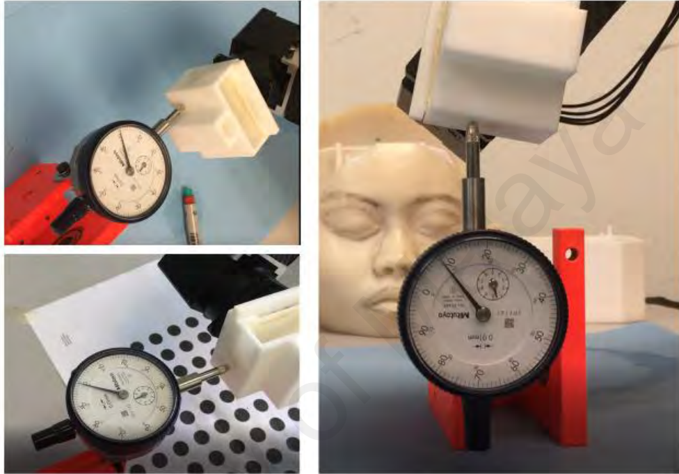
Figure 5.5 using a dial indicator with 0.01mm resolution to calculate repeatability in X,Y and Z at one point of the robot's workspace.
