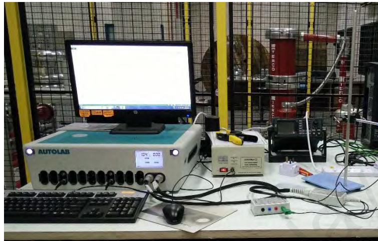
Figure 3.9: The Metrohm potentiostat for FDS and I-V measurements
