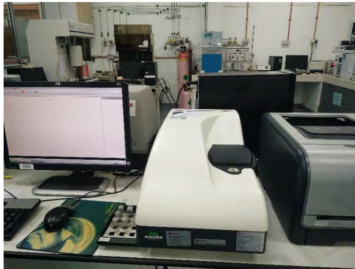
Figure 3.8: A Malvern Zetasizer instrument for DLS measurement
