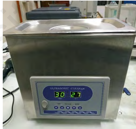
Figure 3.5: Ultrasonic bath to produce homogenous dispersion
