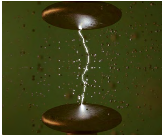
Figure 2.14: Conductive path due to micro-bridging formation (Peppas et al., 2016)
