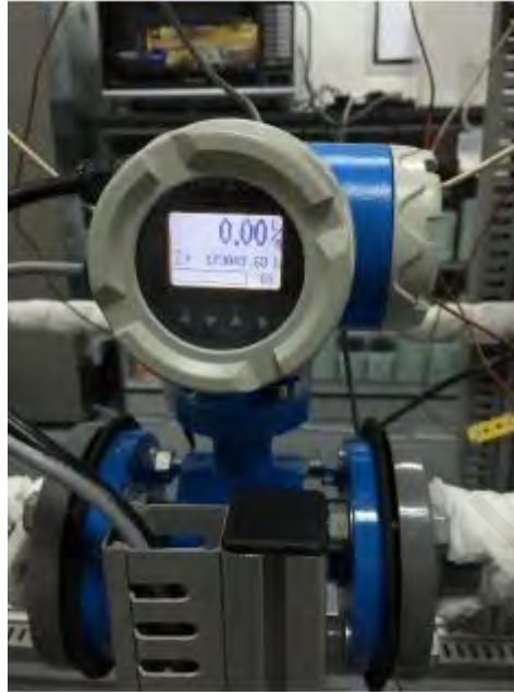
Figure 3. 10: Photograph of the electromagnetic flow meter
