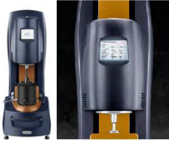
Figure 3. 21: A photograph of the HR-1, Discovery Hybrid Rheometer
