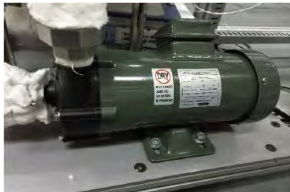
Figure 3. 8: photograph of the magnetic gear pump
