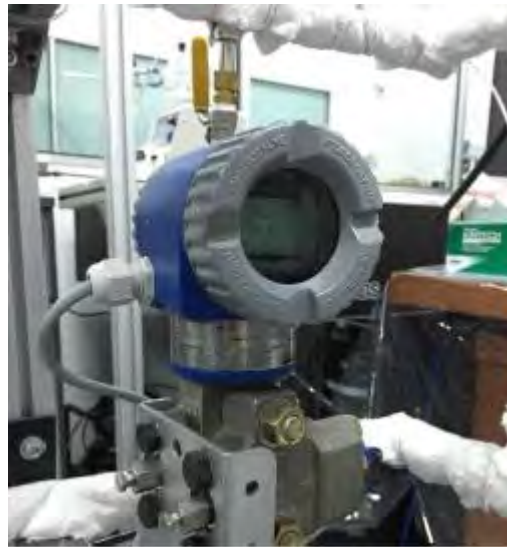
Figure 3. 11: Photograph of the Differential Pressure Transducers
