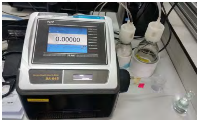
Figure 3. 18: Photograph of the KEM Density/Specific Gravity Meter DA-645.
