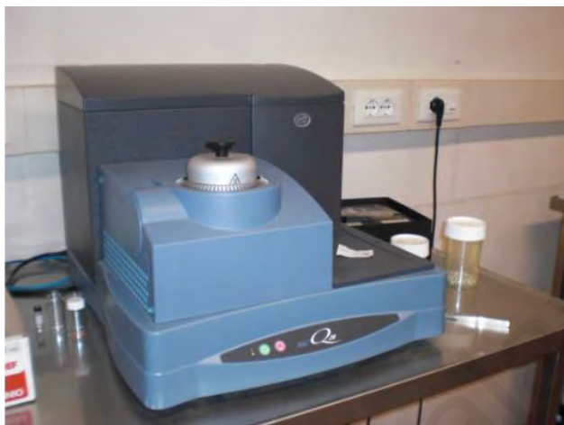
Figure 3. 19: Photograph of the heat flux type differential calorimeter TA DSC Q20.
