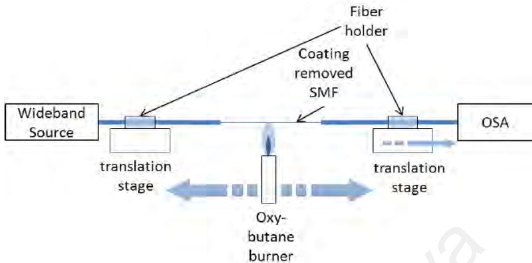
Figure 2.7: Flame brushing rig for tapering fiber (S. et al., 2012).
