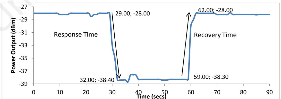
**Figure 4.11:** The response and recovery time of a 2.6  $\mu\text{m}$  tapered fiber coated with PMMA.
