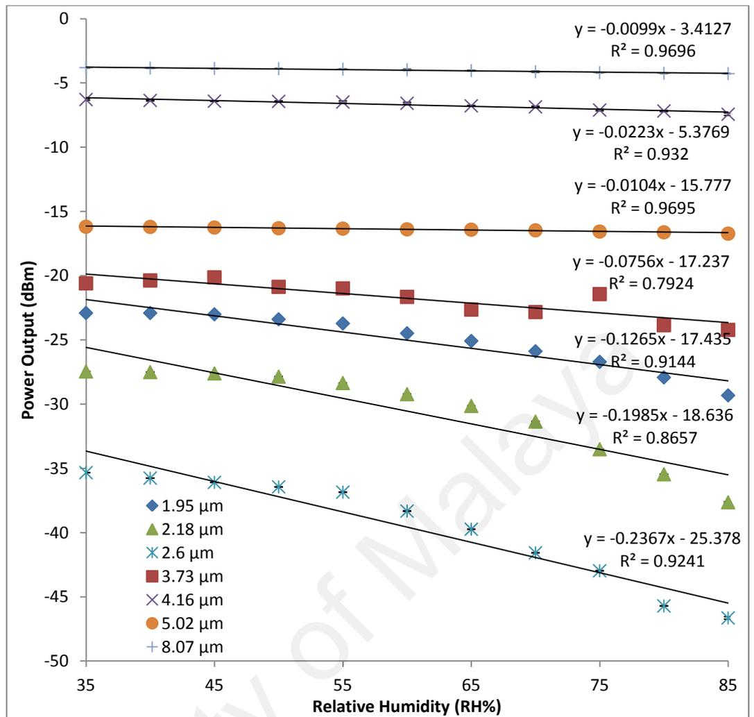
**Figure 3.3: The Power output of various tapering diameters with varying humidity.**
