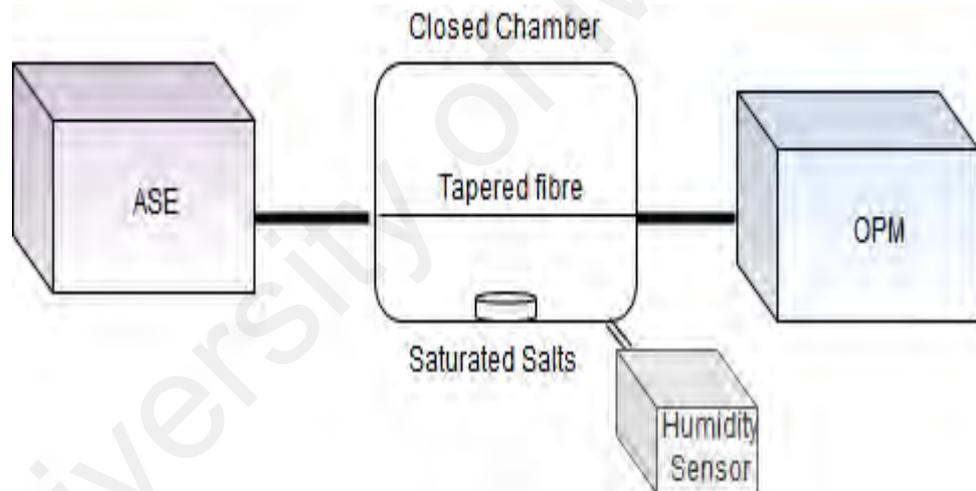
**Figure 3.2: The experiment setup for bare fiber testing**
