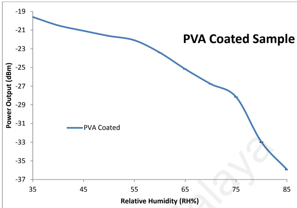
**Figure 4.3: The power output of PVA coated tapered fiber with 2.6  $\mu\text{m}$  diameter with varying humidity.**
