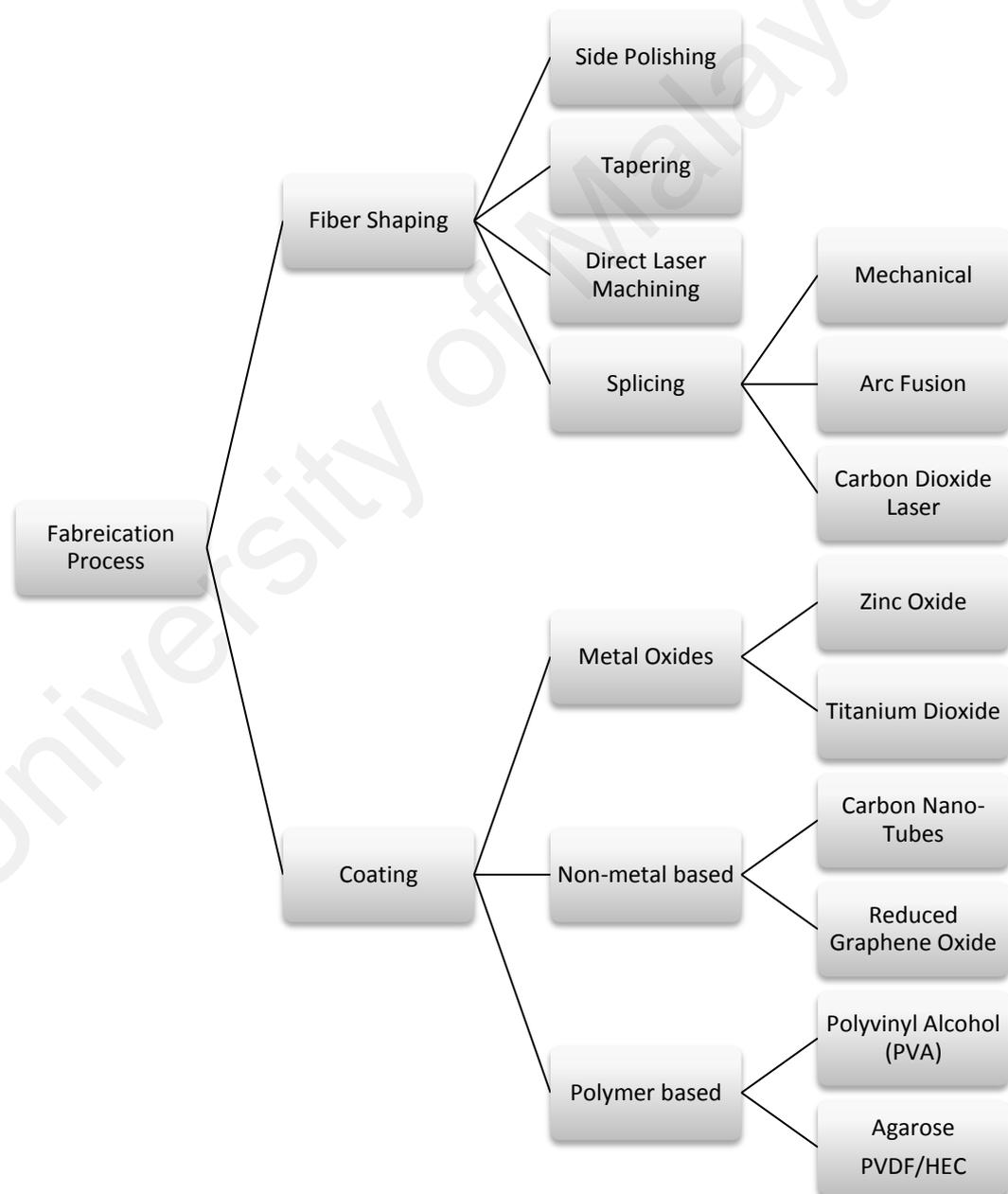
**Figure 2.5: Fiber optics sensors fabrication processes.**
