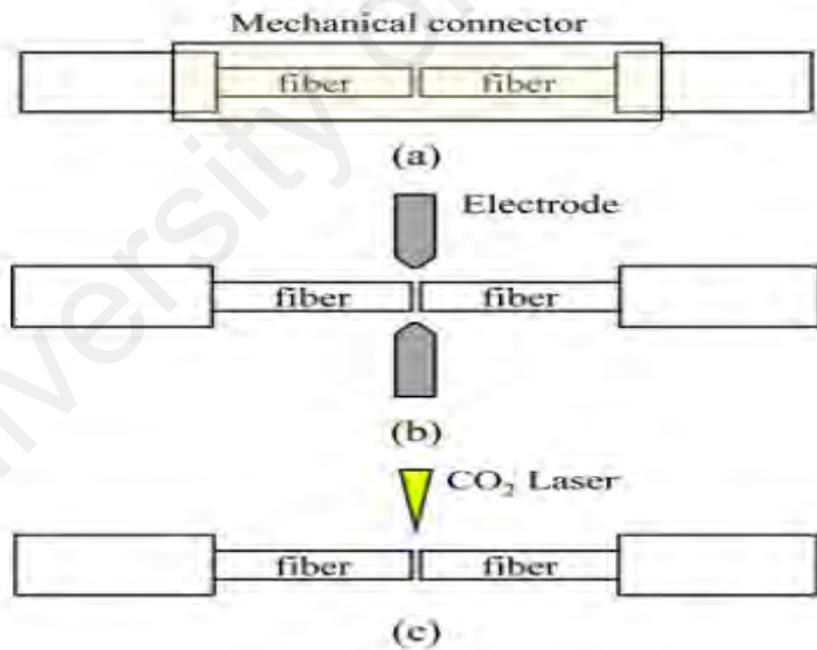
Figure 2.4: Splicing techniques (a) mechanical, (b) arc fusion, and (c) laser splicing (Joe et al., 2018).
