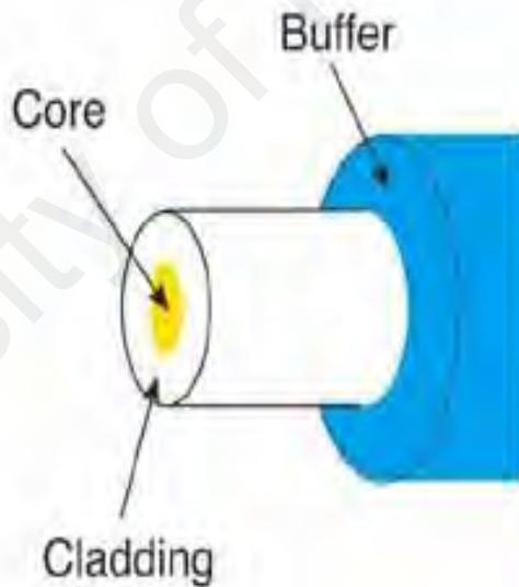
**Figure 2.1: Basic structure of an optical fiber (Thyagarajan & Ghatak, 2007).**
