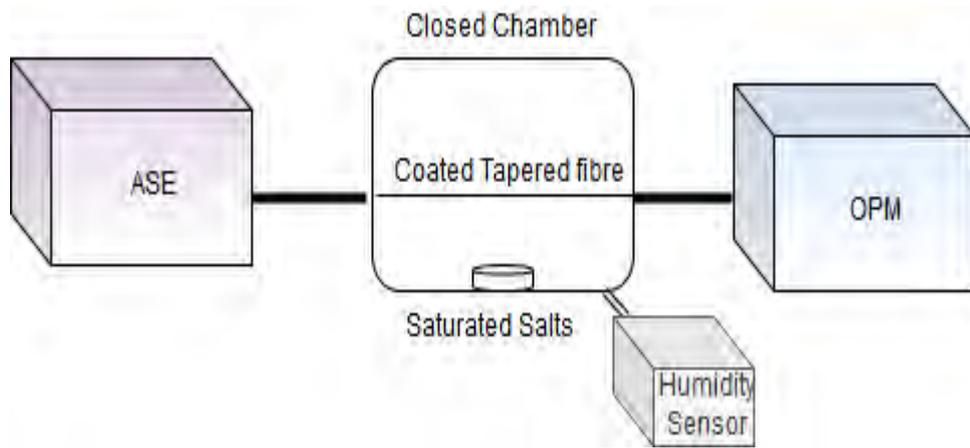
**Figure 4.1: Experiment setup for testing the PVA coated and PMMA coated tapered fiber.**
