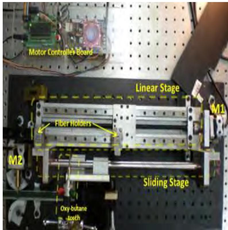
**Figure 3.1: Flame brushing machine (S. W. Harun et al., 2013).**
