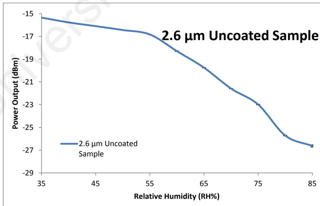
**Figure 4.2: The power output of uncoated tapered fiber with  $2.6 \mu\text{m}$  diameter with varying humidity.**
