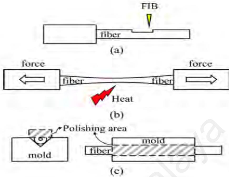
Figure 2.3: Fiber shaping methods (a) Focused ion beam direct machining, (b) tapering and (c) side-polishing (Joe et al., 2018).
