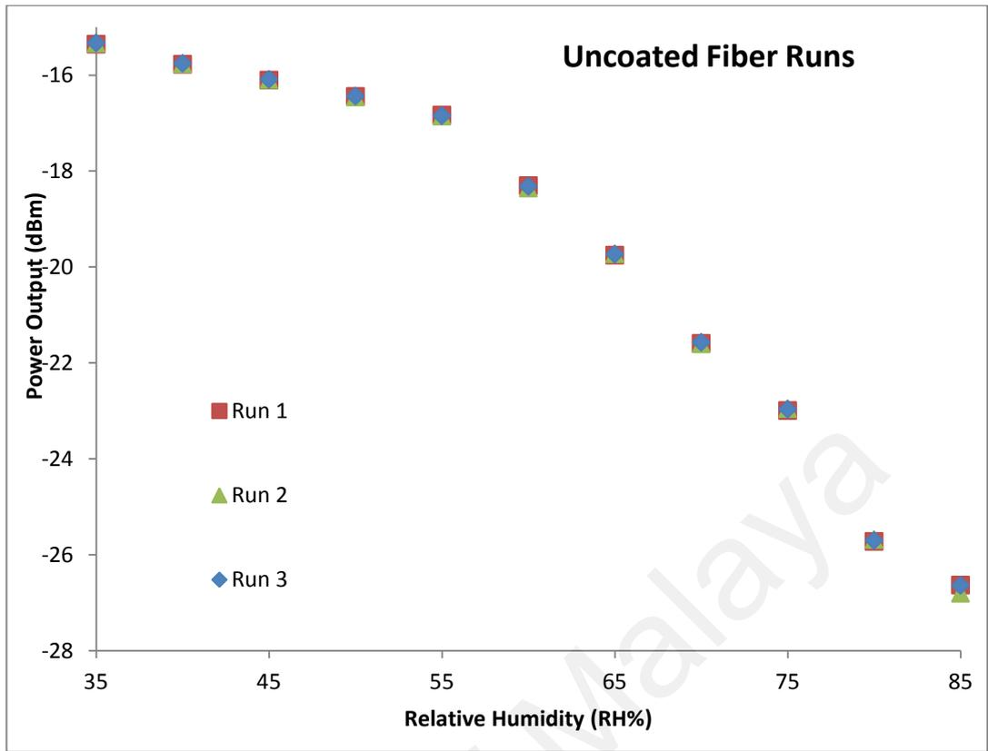
**Figure 4.6: The power output of uncoated tapered fiber in three runs.**
