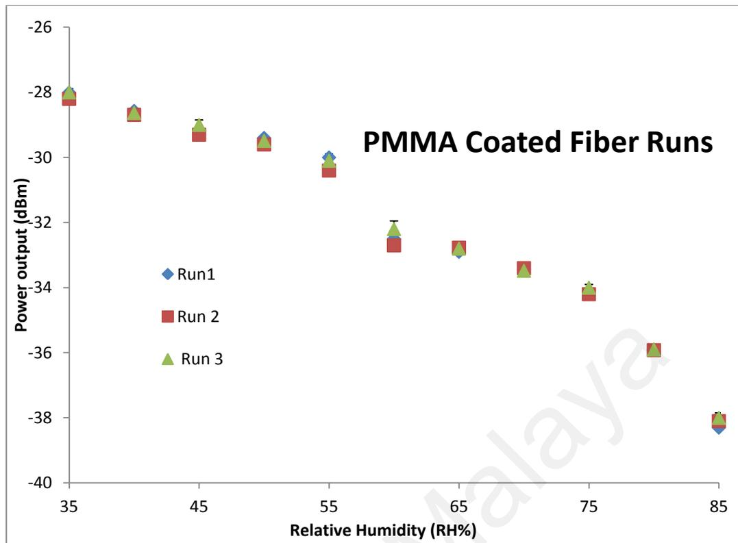
**Figure 4.8: The power output of PMMA coated tapered fiber in three runs.**
