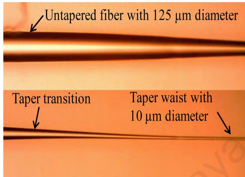
**Figure 2.6: Tapered fiber regions and dimensions (Y. Tian et al., 2011).**
