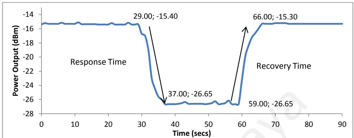
**Figure 4.9:** The response and recovery time of a 2.6  $\mu\text{m}$  tapered fiber.
