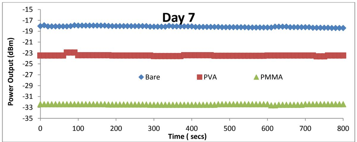
Figure 4.13: Stability of the three samples after seven days.
