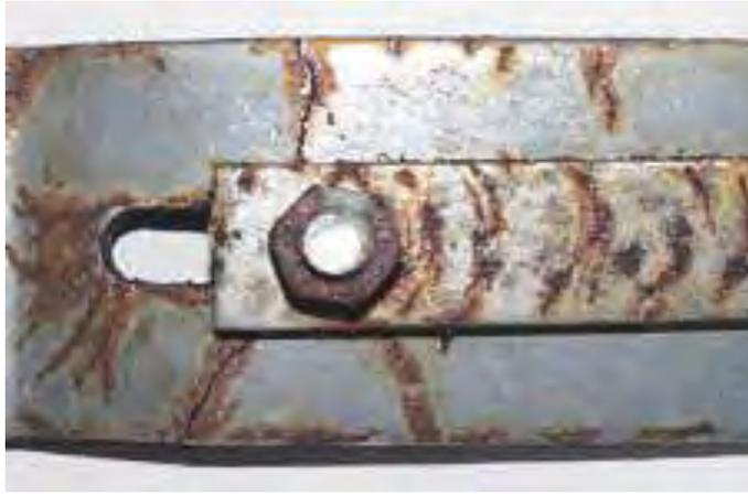
**Figure 2.2: Stress Corrosion Cracking (Nishimura & Maeda, 2004).**
