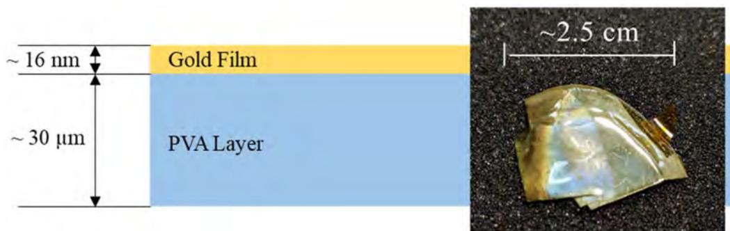
**Figure 3.4: Illustration on thickness of the gold thin-film (Inset) Real image of the gold thin-film**
