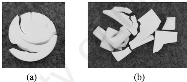
**Figure 4.3: Example of samples crack after microwave sintering with (a) four susceptors, (b) three susceptors.**
