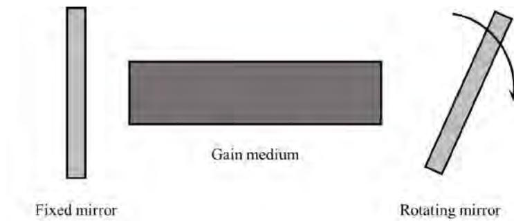
**Figure 2.4: Pulsed laser based on rotating mirror**
