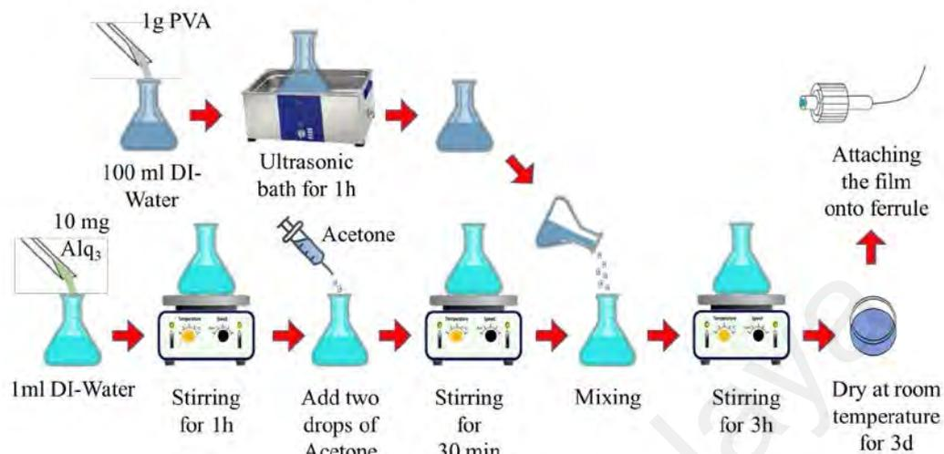
**Figure 3.9: The fabrication process of Alq<sub>3</sub>: PVA thin-film**
