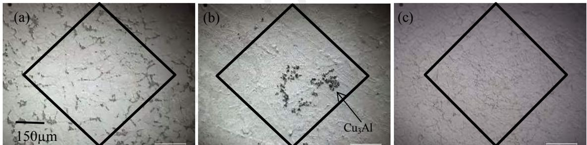
**Figure 4.40** Illustration of Vickers hardness indentation on (a) SAC, (b) SAC+0.5Al and (c) SAC+0.5Zn.
