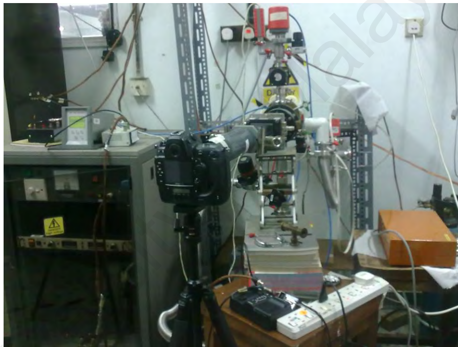
Figure 3.1: The pulsed capillary discharge system at the Plasma Technology Research Centre, University Malaya (UMCD)
