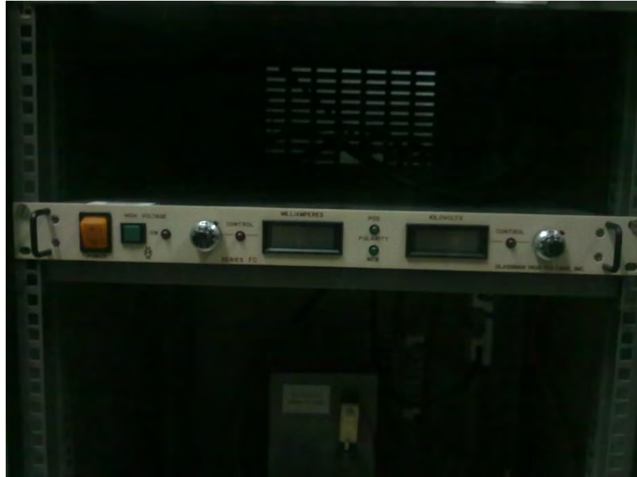
Figure 3.3: High voltage charger
