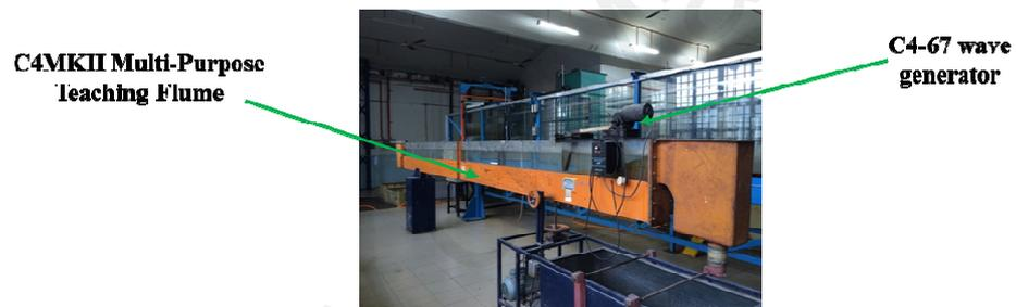
Figure 4.2: SMS wave gauge experimental setup and photo image of the wave maker flume (C4MKII-5.0M Multi-Purpose Teaching Flume mounted with C4-67 wave generator)
