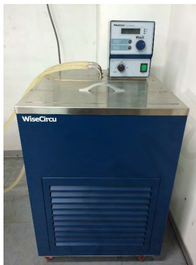
Figure 3.13. Photograph of the Refrigerated Bath Circulators
