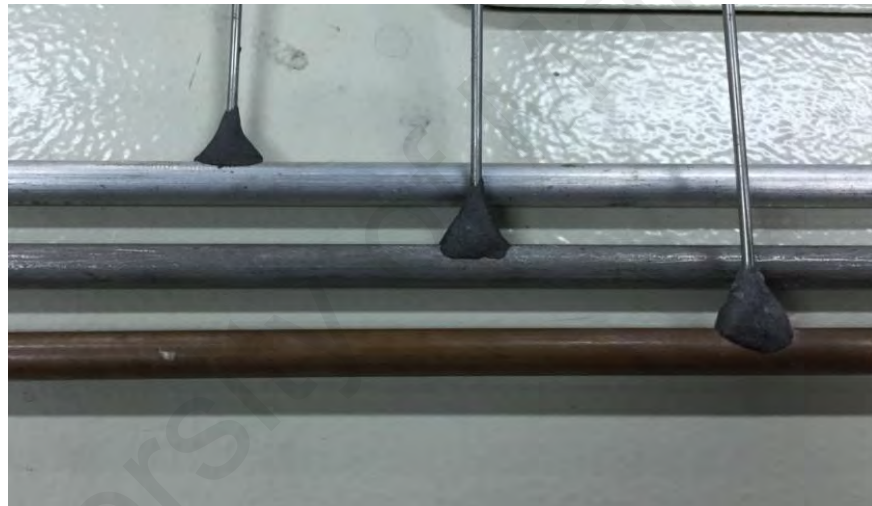
Figure 3.6. Shows the different test sections diameters of stainless steel (2mm, 4mm and 15mm)
