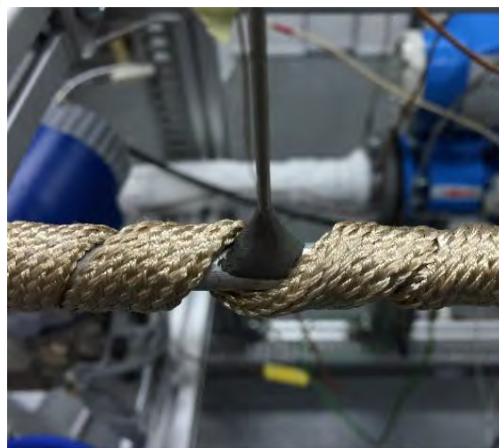
Figure 3.16. Photograph of the heater around the test section
