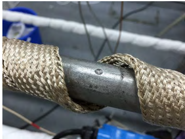
Figure 3.21. Photograph of the groove on a test section
