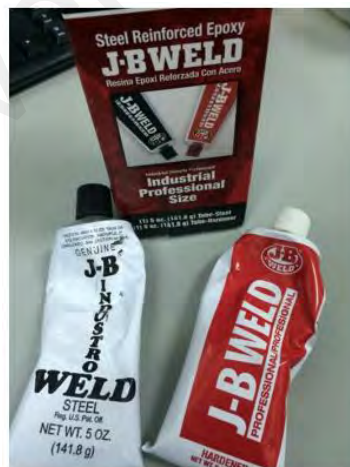
High temp. Epoxy up to 200°C
