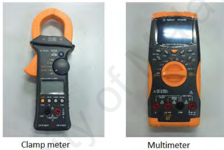
Figure 3.14. Photograph of the Digital Voltmeter and clamp meter
