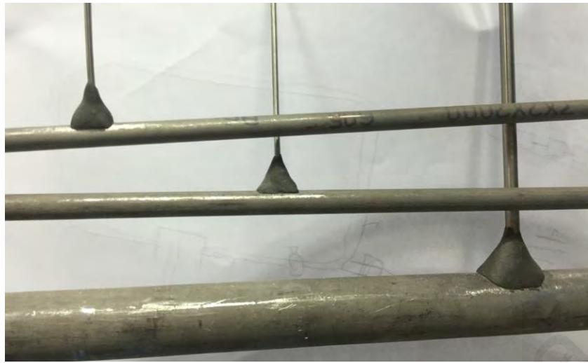
Figure 3.6. Shows the different test sections diameters of stainless steel (2mm, 4mm and 15mm)
