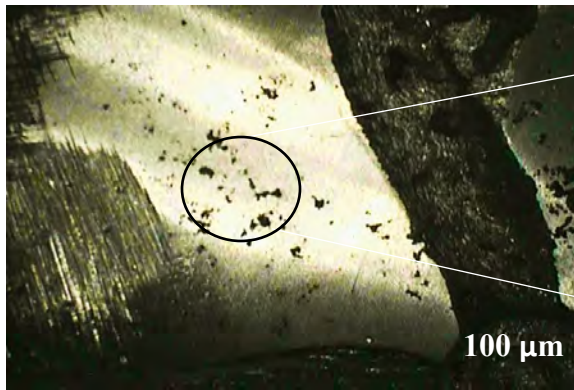
Fig 4.1 Pin Hole defect at 10x Zoom (Sometch)
