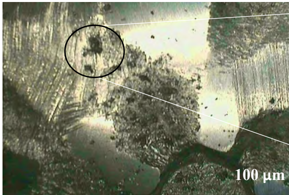
Fig 4.3 Blow Hole defect at 10x Zoom (Sometch)
