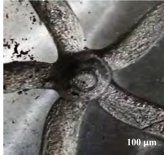
Fig 4.7 Stepping Error at 10x
