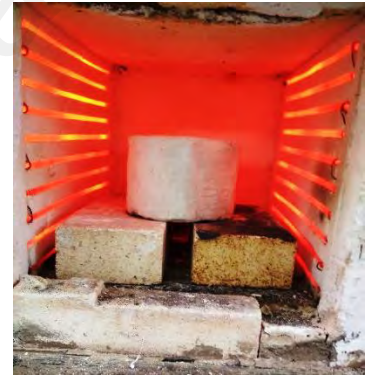
Fig 3.12 Dewaxing of PLA part
