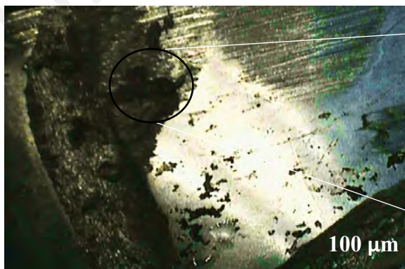
Fig 4.5 Hot tear Defect at 10x (Sometch)
