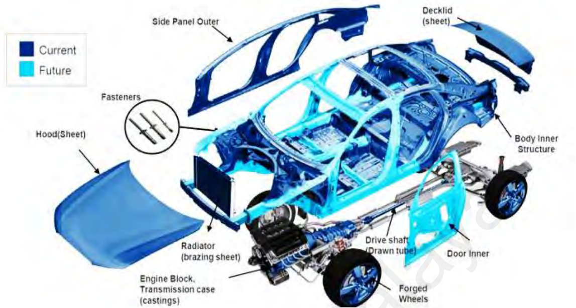
Fig 5.2 Automotive parts produced by Metal Injection Molding (Ludmila, 2012)
