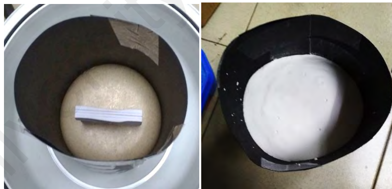
Fig 3.10 Pouring into paper based flask
