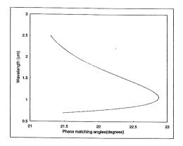
Fig. 2.1 Tuning curve for 532nm pumped BBO parametric oscillator.
