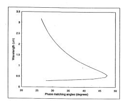
Fig. 2.2 Parametric tuning curve for 266nm pumped BBO OPO
