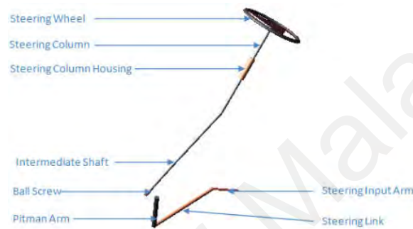
Figure 3-6: Sample MSC.ADAMS Steering System
