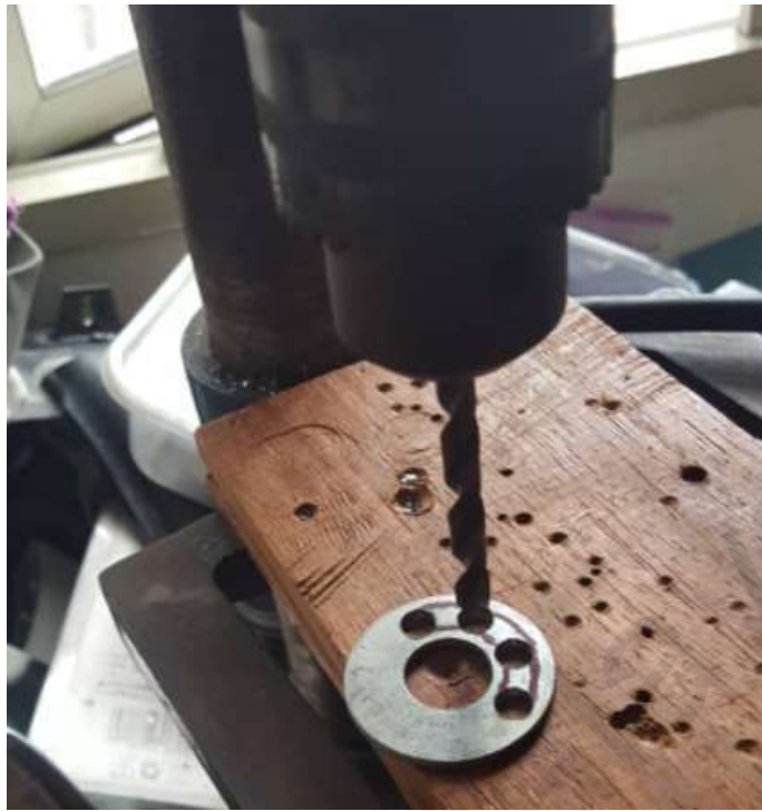
Figure 3-12: 4x Holes Being Drilled Using a Bench Drill
