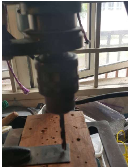
Figure 3-7: Drilling a Hole on the Cantilever Beam for the Asymmetrical Disc
