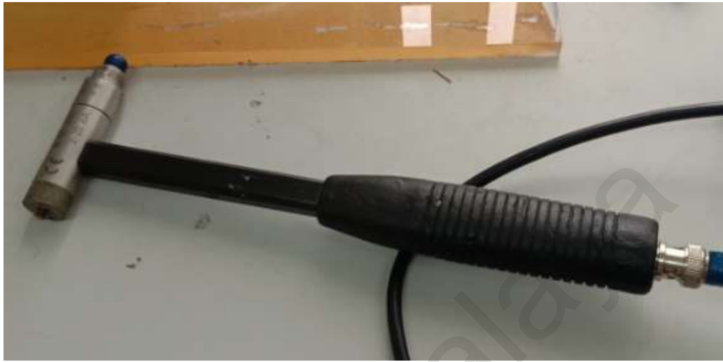
Figure 3-19: Small Hammer Used to Deliver an Impulse to the System
