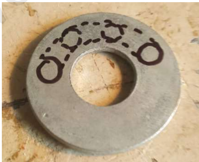
Figure 3-11: Planned Holes on the 36mm Washer
