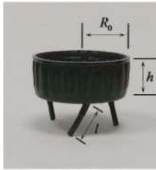
Figure 5-1: A Passive Device that Converts Vibration Motion into Rotary Motion. (Altshuler et al., 2013)
