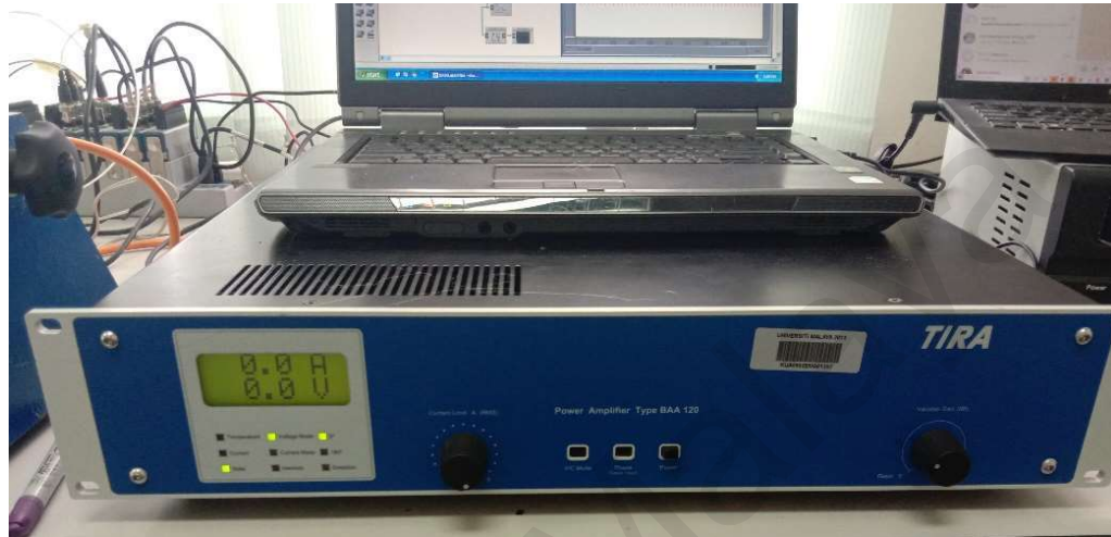
Figure 3-17: Power Amplifier Used to Drive TiraVib Shaker
