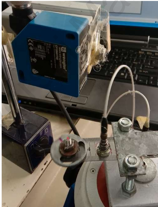
Figure 3-21: Laser Displacement Sensor Measuring Displacement at Tip of Bolt
