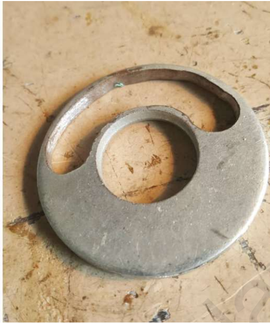
Figure 3-14: Asymmetrical Disc Formed After 4 x Holes Are Joined Together
