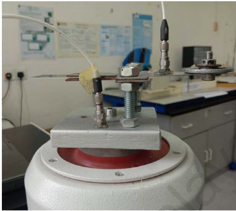
Figure 3-15: Installation of Testing Apparatus on top of TiraVib™ Shaker
