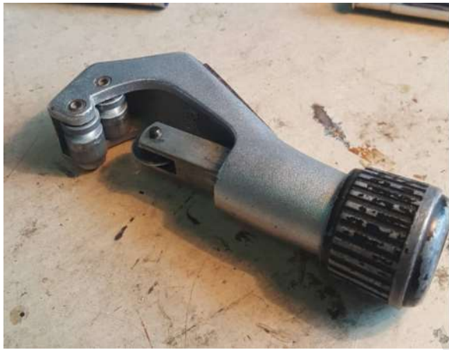
Figure 3-8: Rotary Pipe Cutter Used to Cut the Spacer
