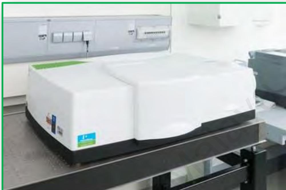
**Figure 3.9:** Perkin Elmer LAMBDA 1050 UV-Vis spectrophotometer
