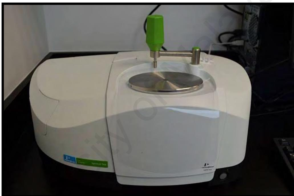
**Figure 3.10.** Perkin Elmer FT-IR spectrophotometer
