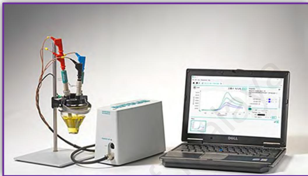
**Figure 3.11:** Metrohm Autolab PGSTAT-204 used to investigate the electrochemical properties of DSSC
