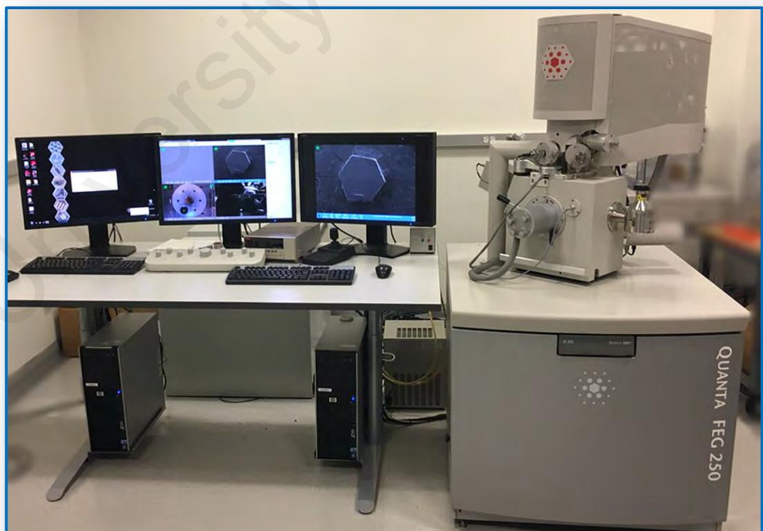
**Figure 3.6:** Field emission scanning electron microscope (FESEM)
