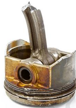
Figure 5.4 : Example of a damaged piston due to corrosion caused by escaped moisture content .
