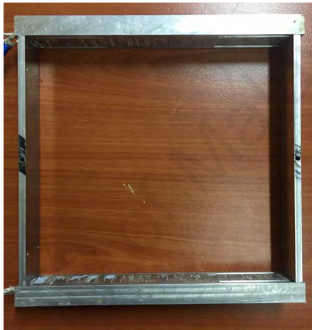
Figure 3.3: Aluminium Heat exchanger housing
