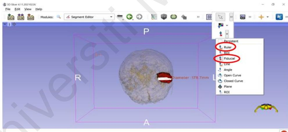
Figure 36: a) The red circle shows fiducial tool to create reference point. b) The red circle shows ruler tool to measure length between two reference points
