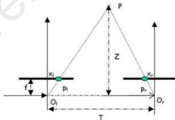
Figure 10 shows two different projections of point  $P$  on image of  $P_1$  and  $P_r$ .  $O_1$  and  $O_r$  explained the coordinate of two cameras
