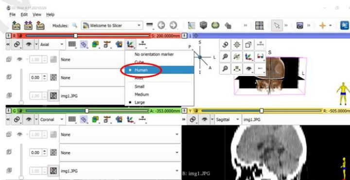
Figure 29: The red circle shows human widget that will allow user view direction view of 3D model.
