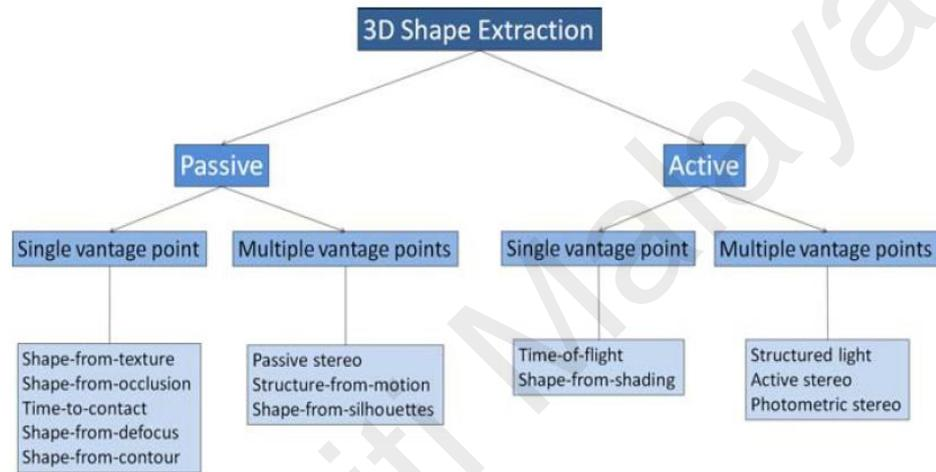
Figure 3 Three-dimensional acquisition methods
