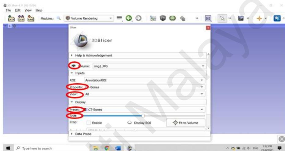
Figure 28: a) The red circle shows eye symbol to allow 3D model to display on the scene. b) the red circle shows property of the volume scene. c) The red circle shows view mode for the scene. d) The red circle shows type of pre-set selected for 3D model display in the scene. e) The red circle shows the shift level for the 3D model.
