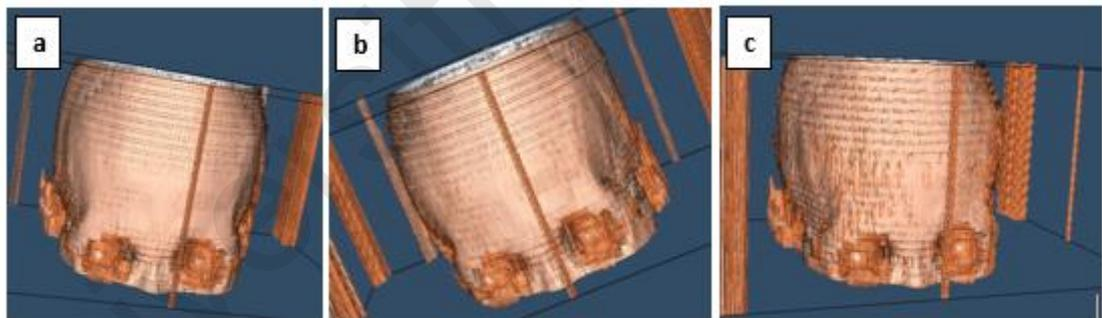
Figure 53: The diagram shows different value of skin extraction result. A) The skin extraction value is 20 shows smooth external surface. b) The skin extraction is 10 and c) the skin extraction is 5 have rougher external surface.
