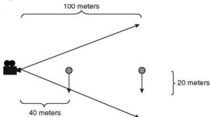
Figure 11 shows the object with 100m away is moving 20m downward and still located in the observer's field of view while the object with 40m away is moving with the same displacement disappeared from the field of view
