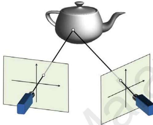
Figure 4 Passive triangulation
