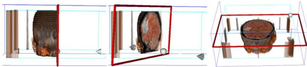
Figure 41: Result of volume rendering with additional features. The diagram shows a red plane with white arrow that allow user to view cross-section of the model.
