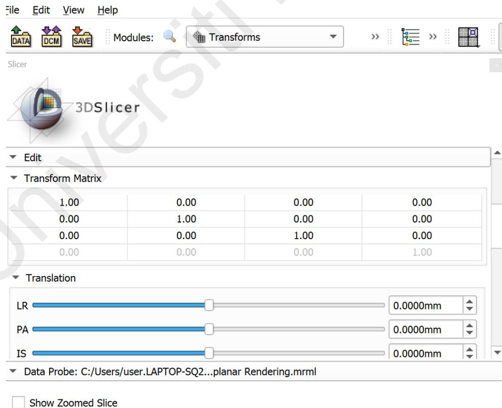
Figure 51: The diagram shows the transform modules in 3D slicer that stores voxel data in 4x4 matrix.
