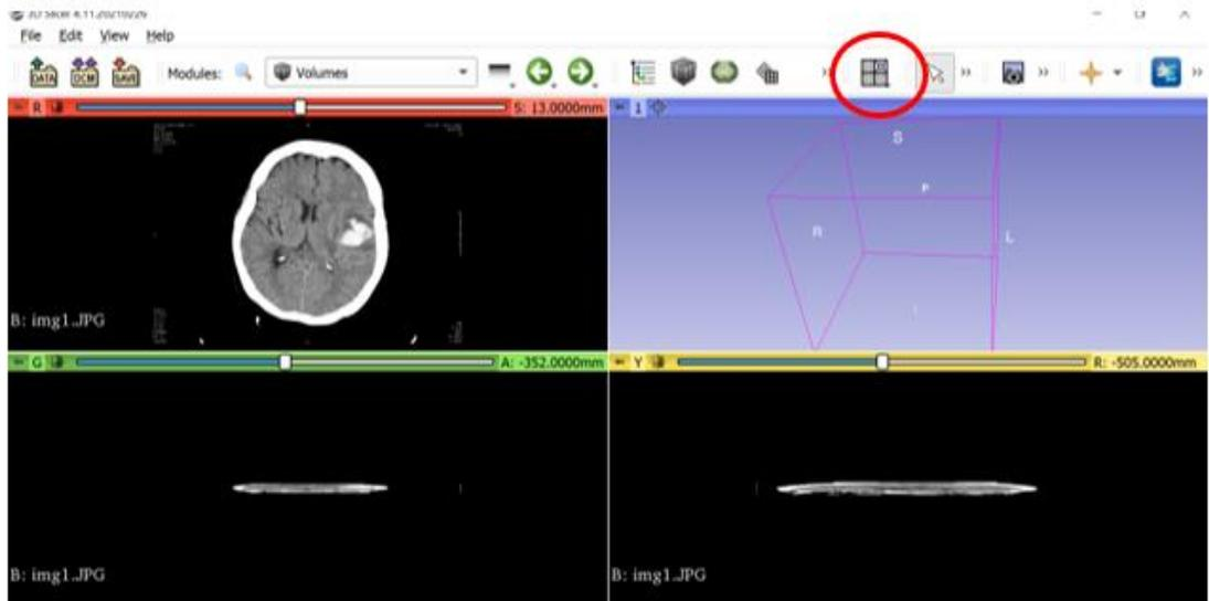
Figure 26: Red circle shows scene widget set as 'four up' scene. Red coloured tab shows axial view, green coloured tab shows coronal view, yellow coloured tab shows sagittal view and blue coloured tab shows volume view.
