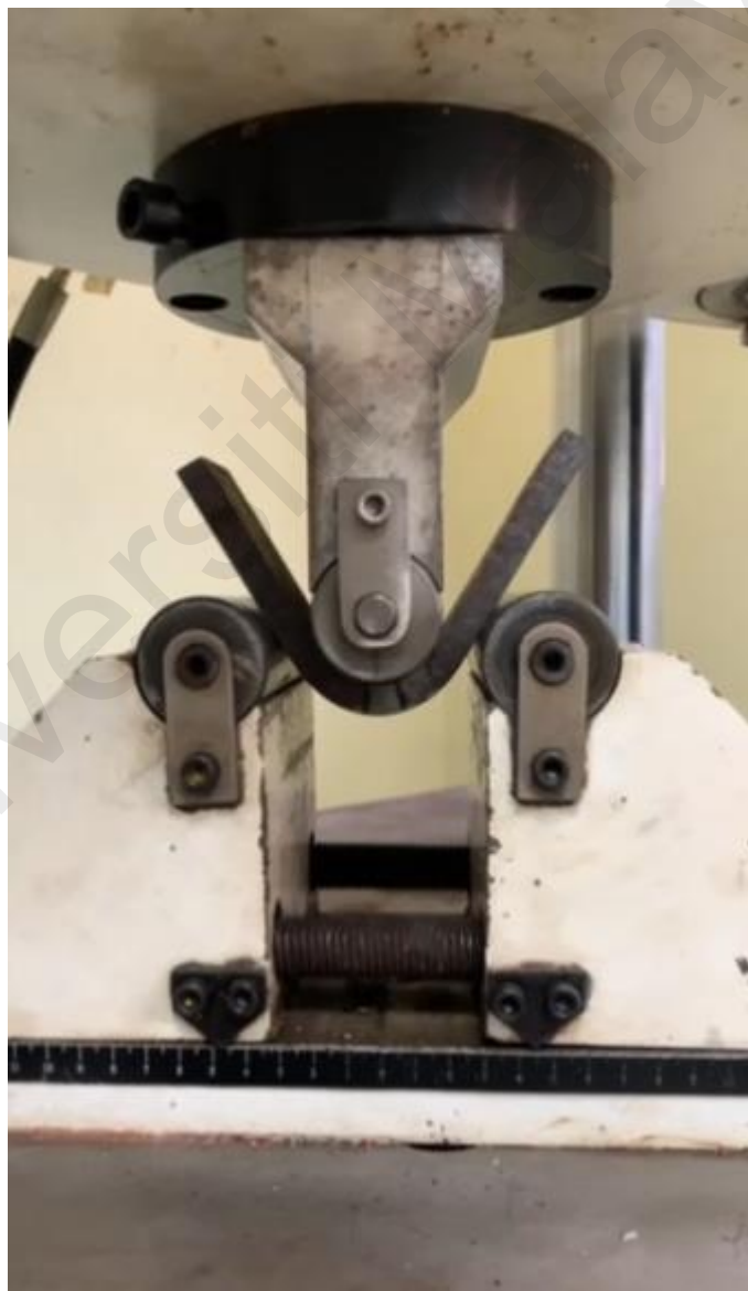
Figure 3.7: Specimen condition while bend test in progress
