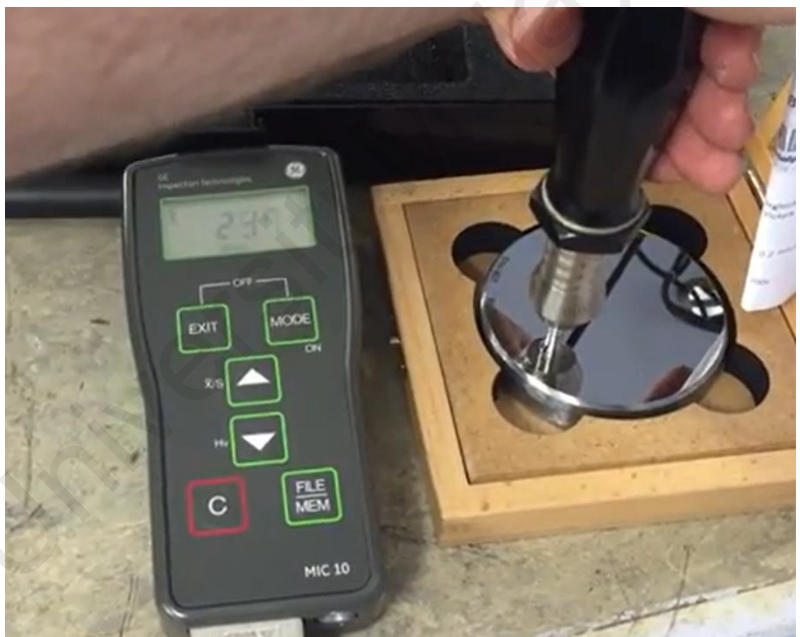
Figure 3.8: Hardness equipment verification before measurement
