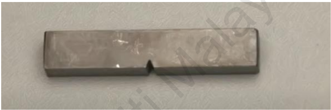
Figure 3.5: Impact test specimen before testing
