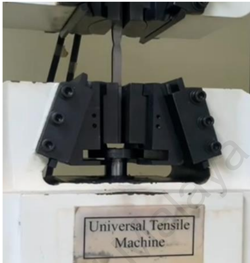
Figure 3.3: Specimen condition while tensile test in progress
