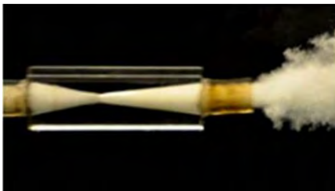
Figure 1.1: Microbubble generation in a venturi tube (Tsuge, 2016).
