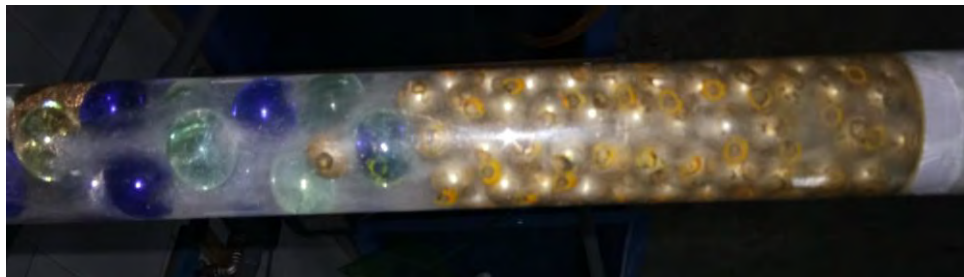
Figure 4.5 Flow condition of two-phase marbles.
