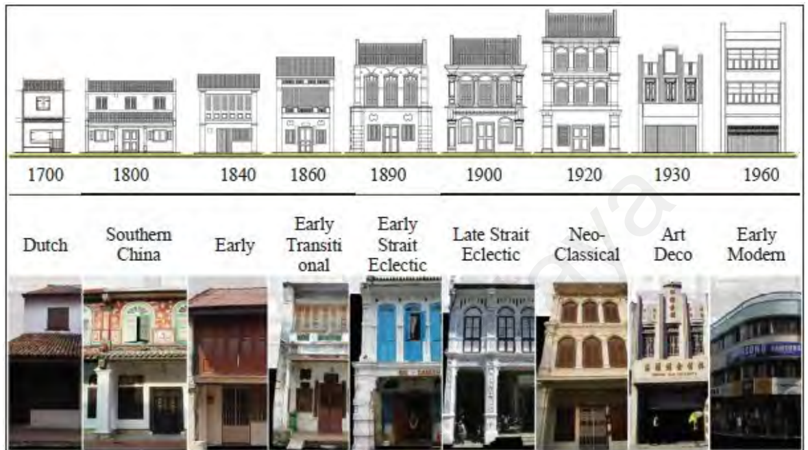
Figure 2.3: Façade of Penang Shophouse in different periods. Source: Noorfadhilah Mohd Baroldin
