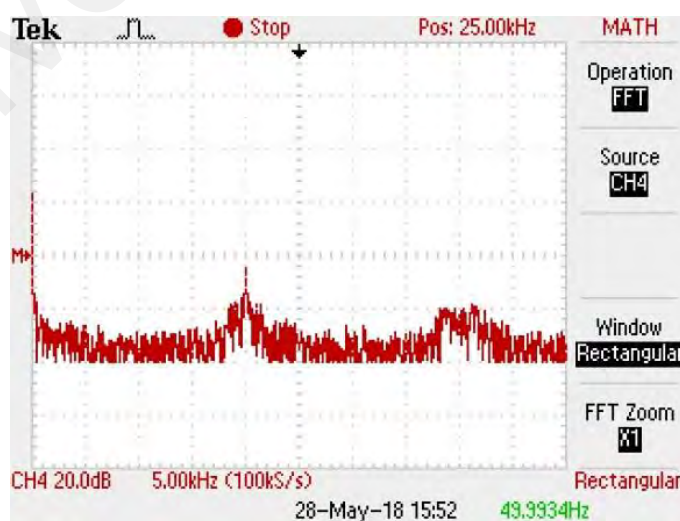
Figure 5.40: FFT of Output-Voltage for Balanced condition
