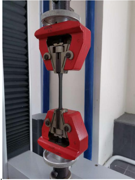
Figure 3.9 The Universal Testing Machine used for tensile test from MS INSTRUMENTS (SEA) SDN.BHD
