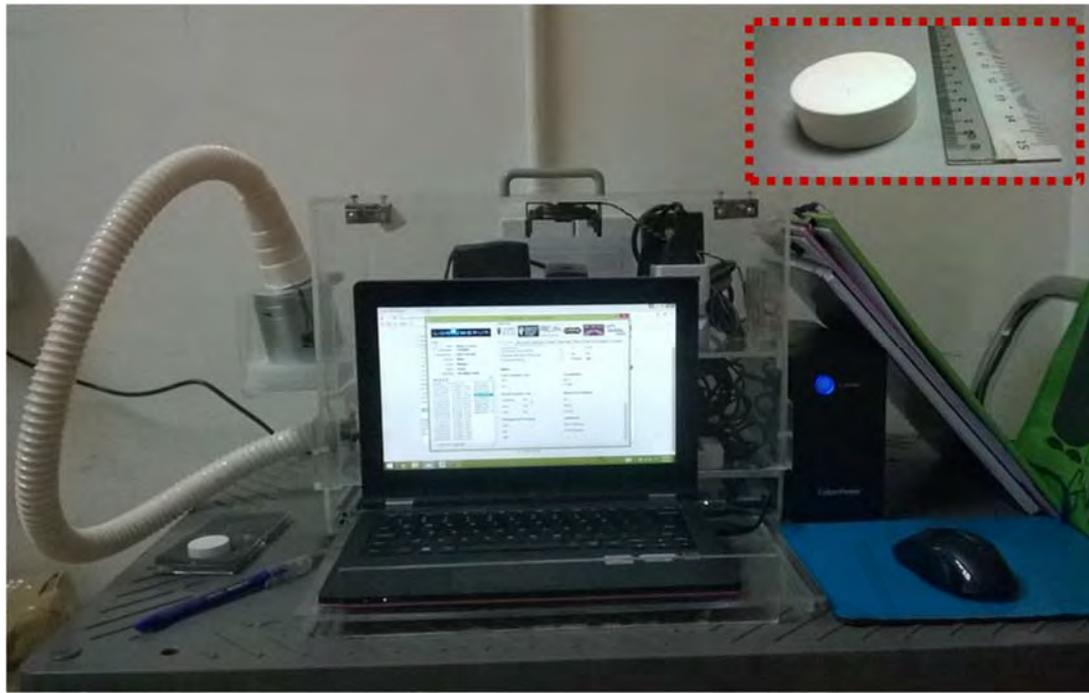
Figure 3.7: Setup in secondary triage area. The inset is the reflection standard.
