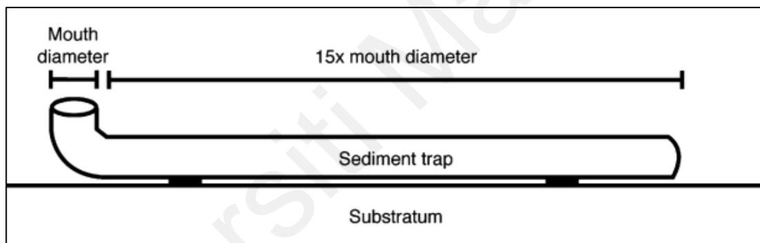
**Figure 3.2: Diagram of sediment trap used by following the design for intertidal sampling, with height-to-mouth diameter (H/D) ratio of 15cm (Schiel et al., 2006).**
