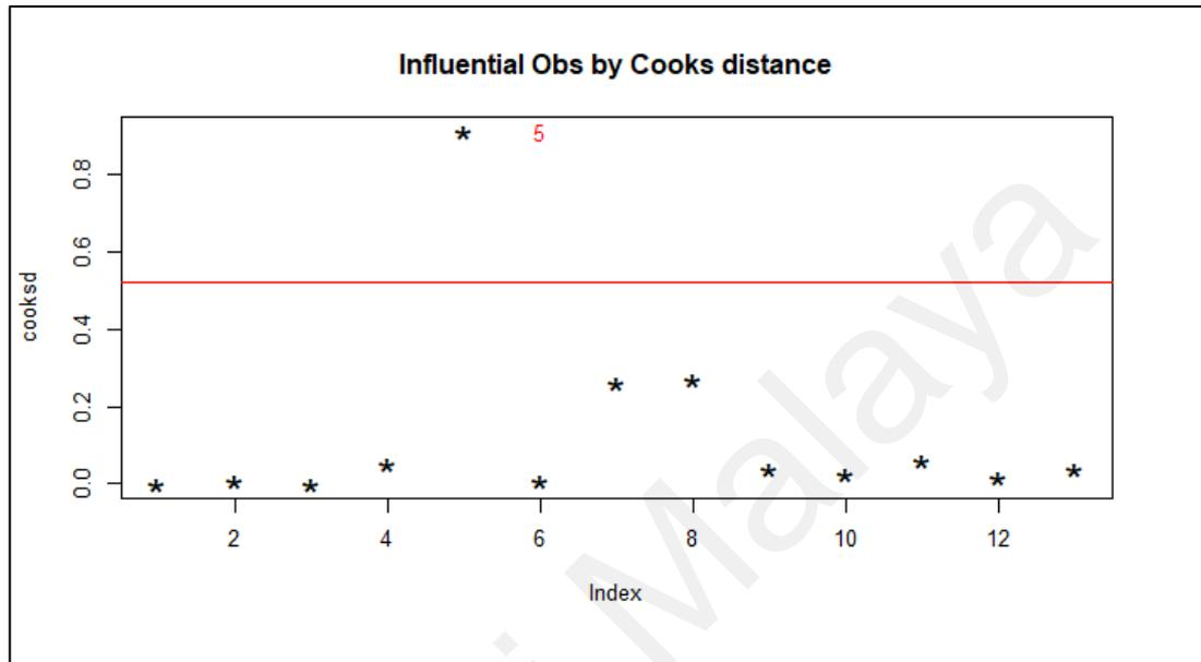
**Figure 4.5:** Plot graph shows the index of Cook's Distance calculated from the observed data. Any observation above the red line is considered highly influential to the model.
