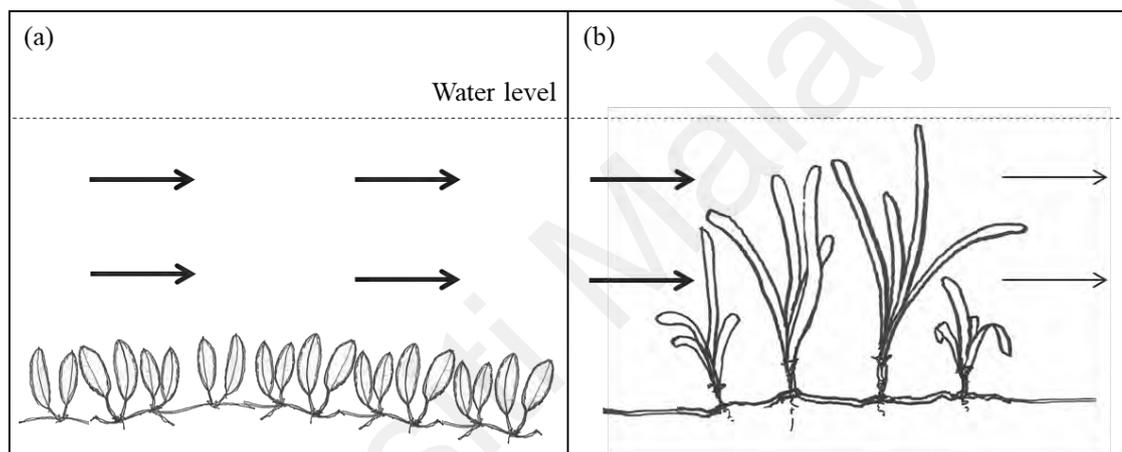
**Figure 2.3: Current flow comparison between two different seagrass canopy height in water column. Flow reduction in low canopy seagrass (a) that occupies a small fraction of water column is less efficient than high canopy seagrass (b) that occupies the whole water column. Arrows indicate current flow, where thicker arrow shows higher velocity.**
