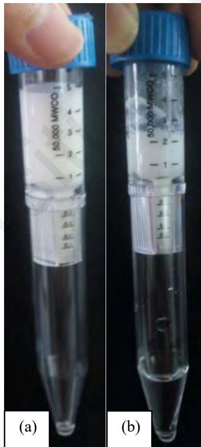
Figure 3.12: (a) Centrifugal filter tube before centrifuge and (b) centrifugal filter tube after centrifuge
