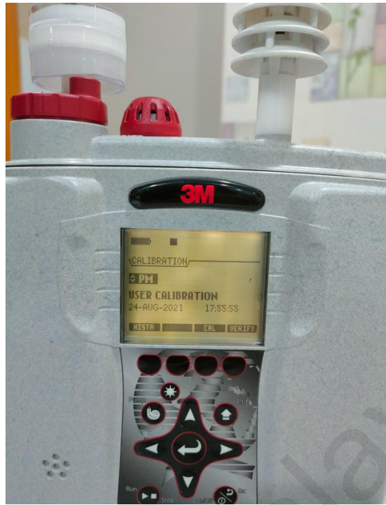
Figure 3. 8: Calibration of EVM using Zero/HEPA filter
