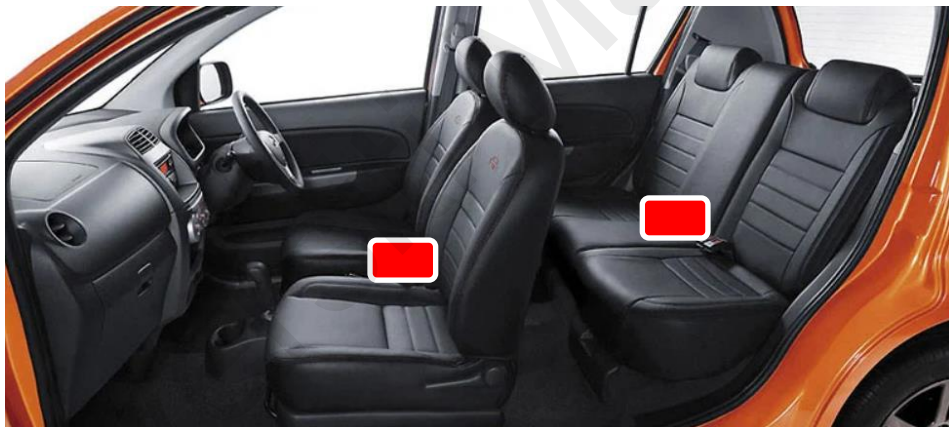
Figure 3. 4: 3M EVM Instrument placement of Perodua Myvi
