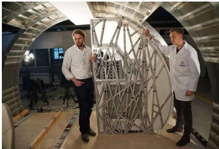
Figure2.4: Large-scale "bionic" cabin isolation structure for Airbus A320 aircraft
