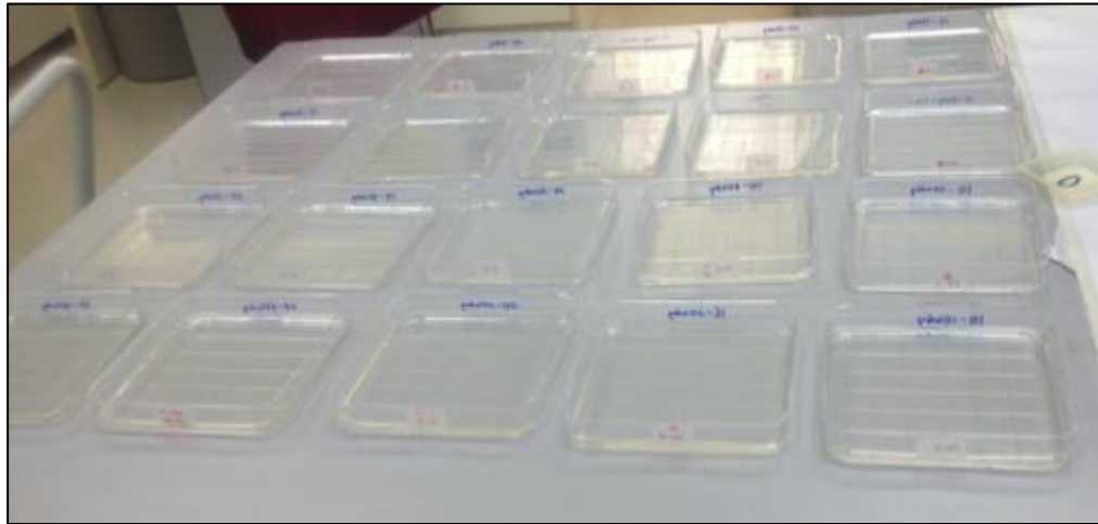
Figure 3.3: CS/PVA polymer blend were casted in the petri dish
