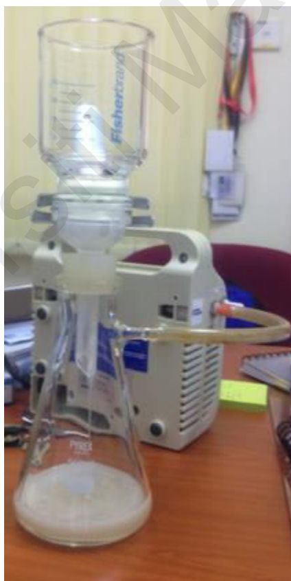
Figure 3.2: Chitosan solution was filtered to remove dust and impurities
