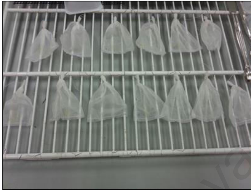
Figure 3.5: Samples in the tea bags after immersion in the water
