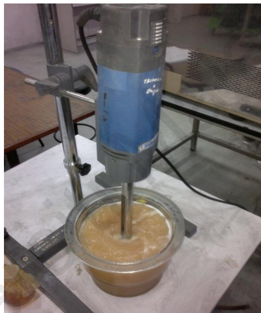
Figure 3.5: Setup for the homogenous fuel blending process
