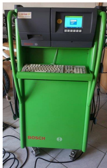
Figure 3.7: BOSCH BEA-350 exhaust gas analyzer
