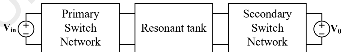
Figure 2.2 A general layout of Non-isolated bidirectional resonant converter
