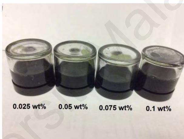
**Figure 4.6: Photograph image of prepared sample of GNP nanofluid after three months**
