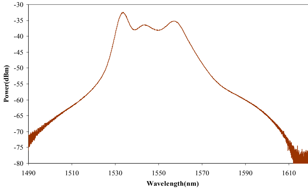
Figure 3.10(a): ASE spectrum of Bi-EDFA
