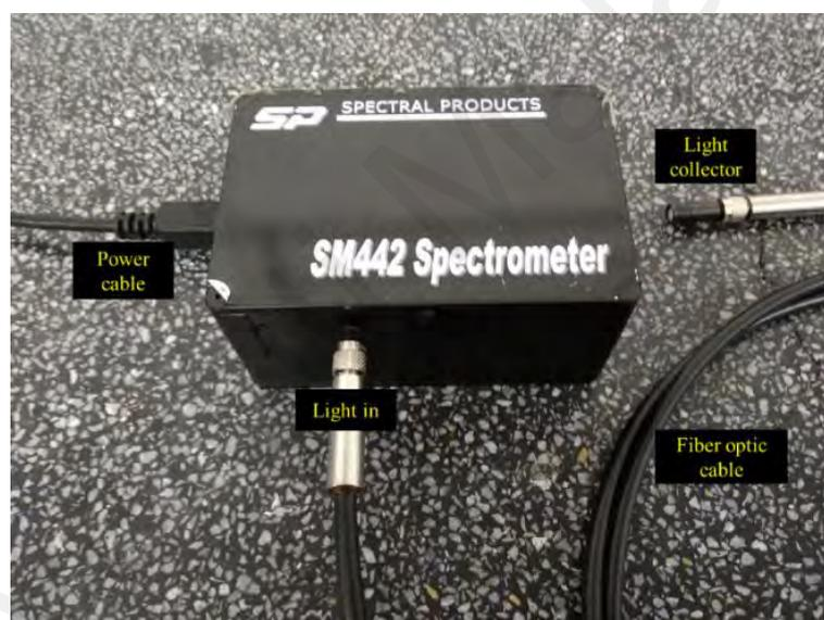
**Figure 3.17:** SM442 Spectrometer connected to fiber optic cable.
