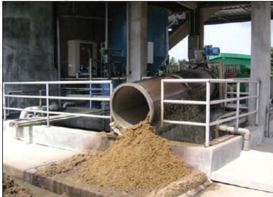
Figure 2.4: Example of Waste Separation Mechanism
