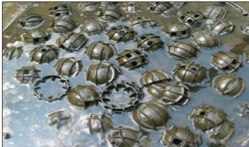
Figure 2.5: Bio-filter Containing Functional Media Balls
