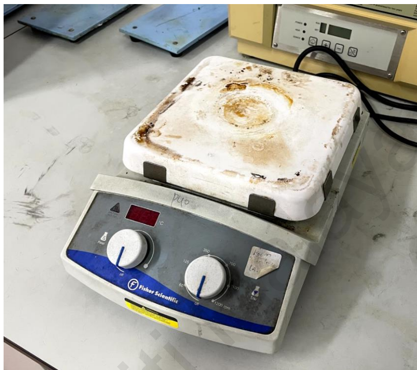
Figure 3.2: Magnetic stirrer hot plate used to mix all the components in the mixture.
