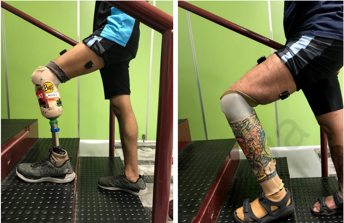
Figure 3.13: Muscles that were targeted above the knee (RF, BF) with (TTAmp S1 & TTAmp S2) during stairs ascending activity
