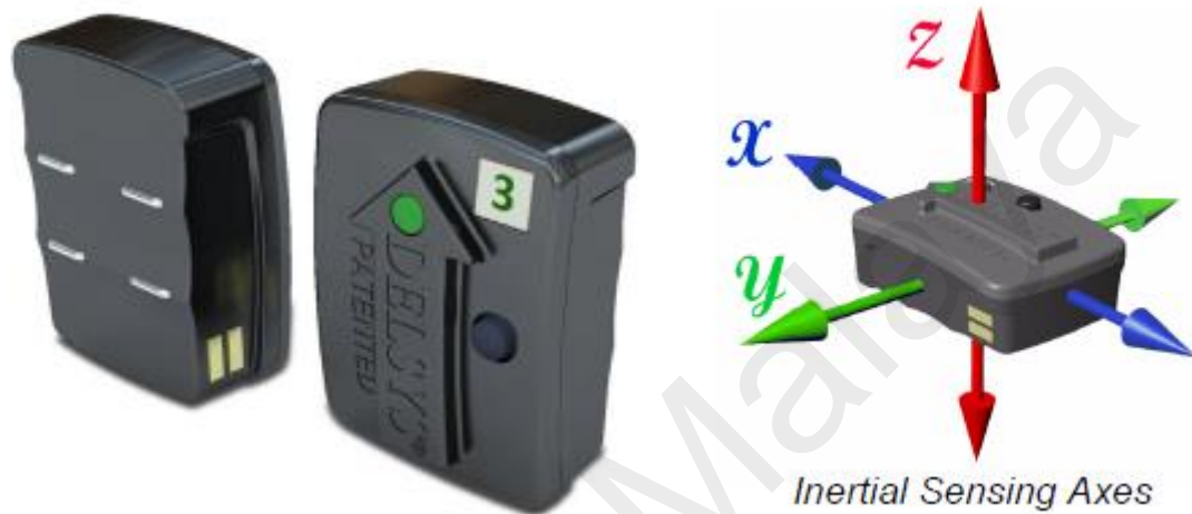
Figure 3.2: Wireless EMG 4-channel sensor (delsys.com, 2018)
