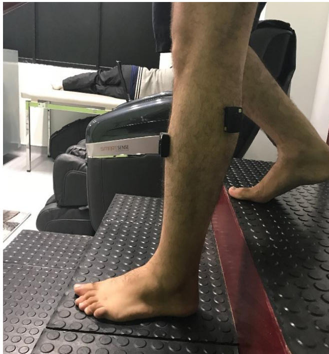
Figure 3.16: Muscles that were targeted below the knee (TA, LG) with male subject during descent stairs
