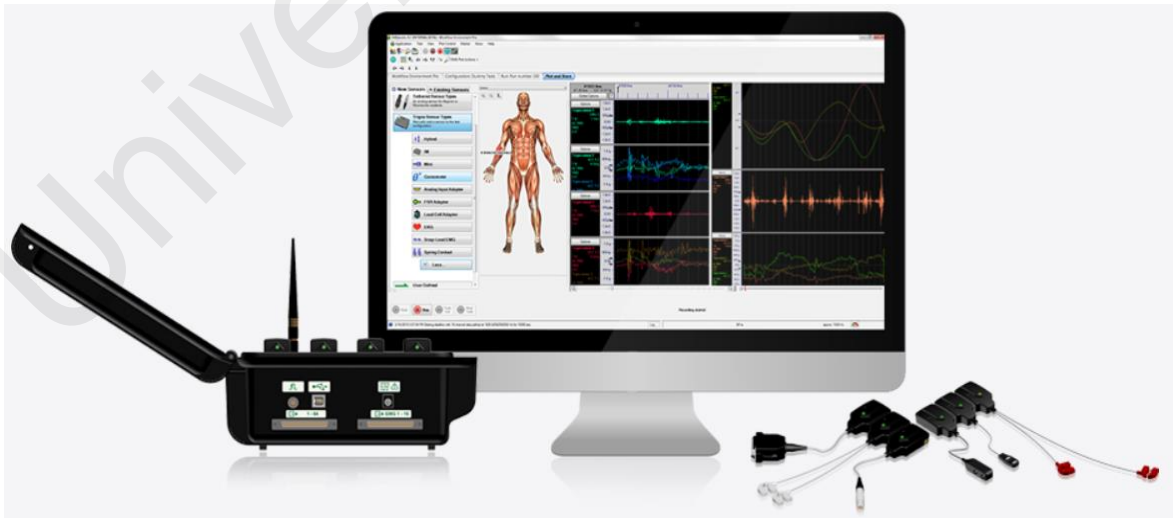
Figure 3.1: DELSYS Trigno™ Wireless EMG device (delsys.com, 2018)
