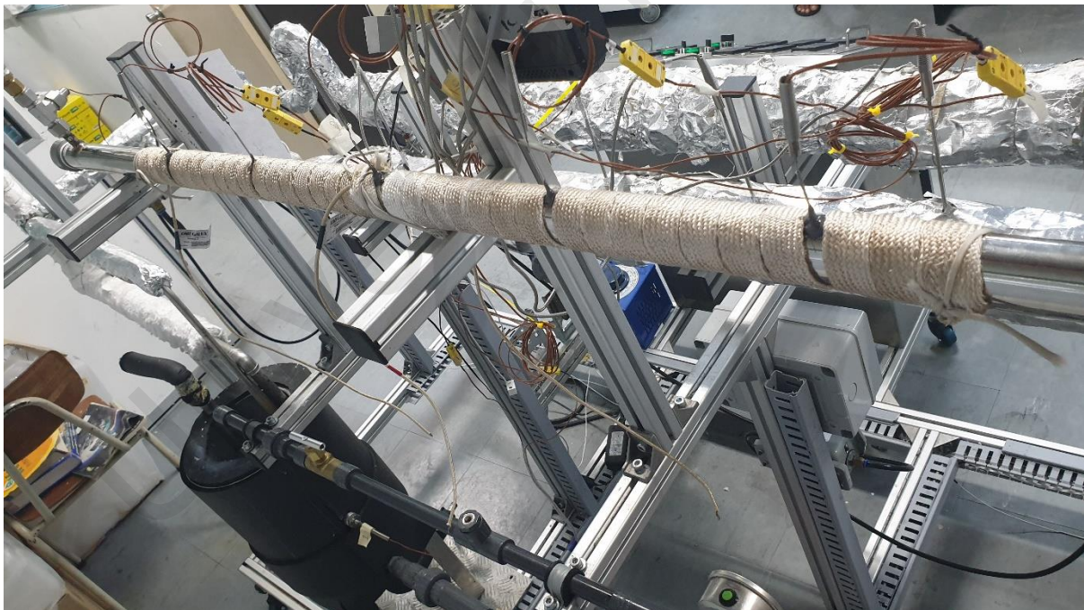
Figure 3. 6: Photograph of Tape heater wrapped along the whole length of the stainless-steel pipe.
