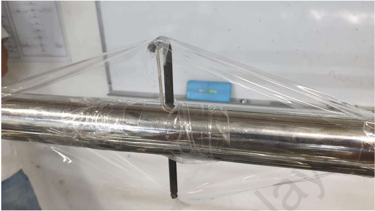
Figure 3. 4: Photograph of thermocouple slot held in place using Allen key and transparent tape.
