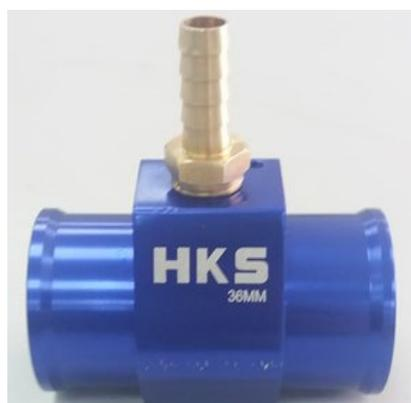
**Figure 3.7: T-junction made from modified HKS coolant hose connector.**
