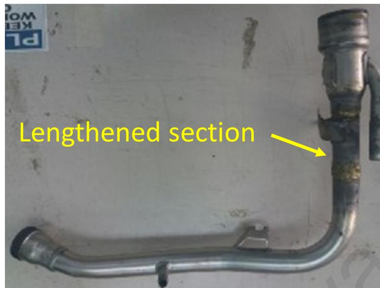
**Figure 3.9: With reference to the original thermostat pipe in Figure 3.8, the pipe near the bypass outlet was lengthened to allow ample clearance to the coolant outlet at the back of the cylinder head.**
