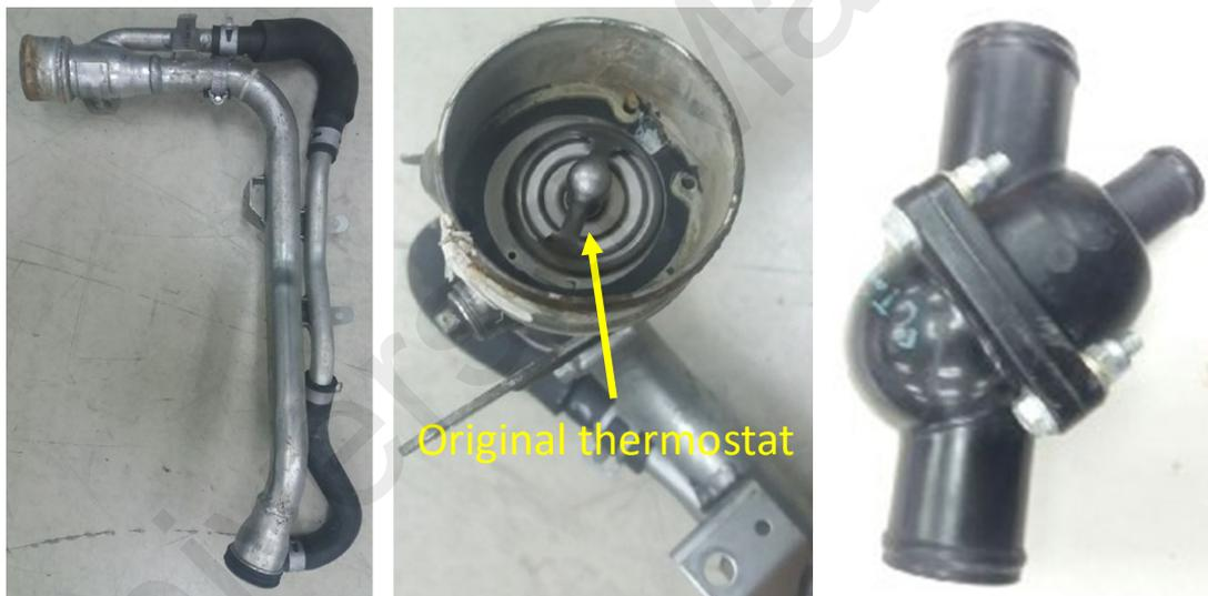
**Figure 3.8: Left photo: Original thermostat pipe. Centre photo: Original thermostat inside the thermostat pipe. Right photo: WTI thermostat housing with the thermostat integrated within the plastic housing.**
