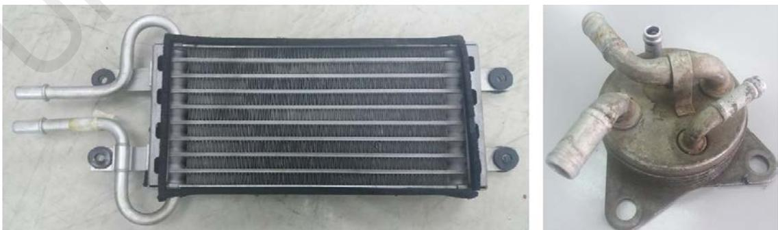
**Figure 3.10: Left photo: The original CVT oil radiator. Right photo: Oil-to-coolant heat exchanger which replaced the original CVT oil radiator.**
