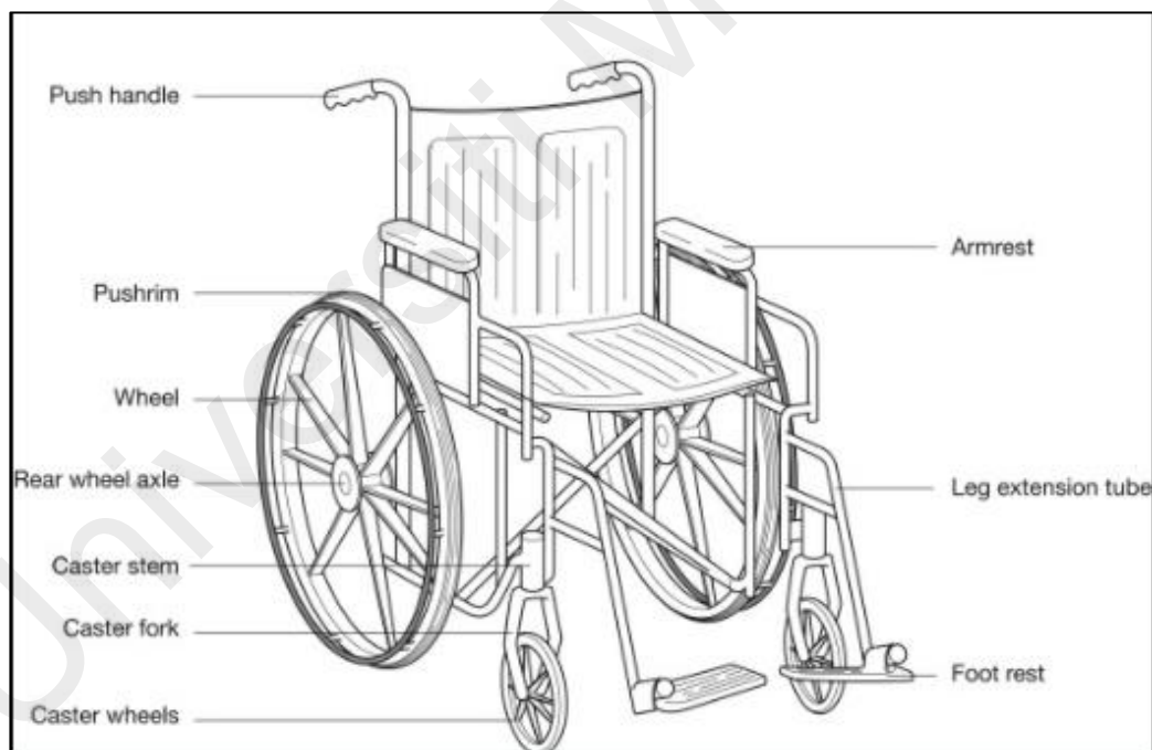
Figure 2.10: The basic wheelchair. Source from Wheelchair and Seating System (M. Koontz et al., 2015).
