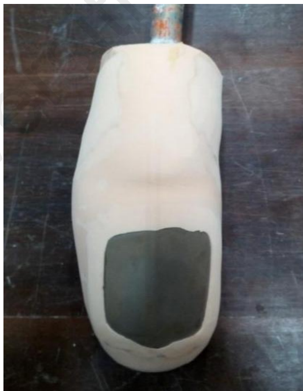
Figure 4.6 Prosthetic liner with polyurethane foam modification
