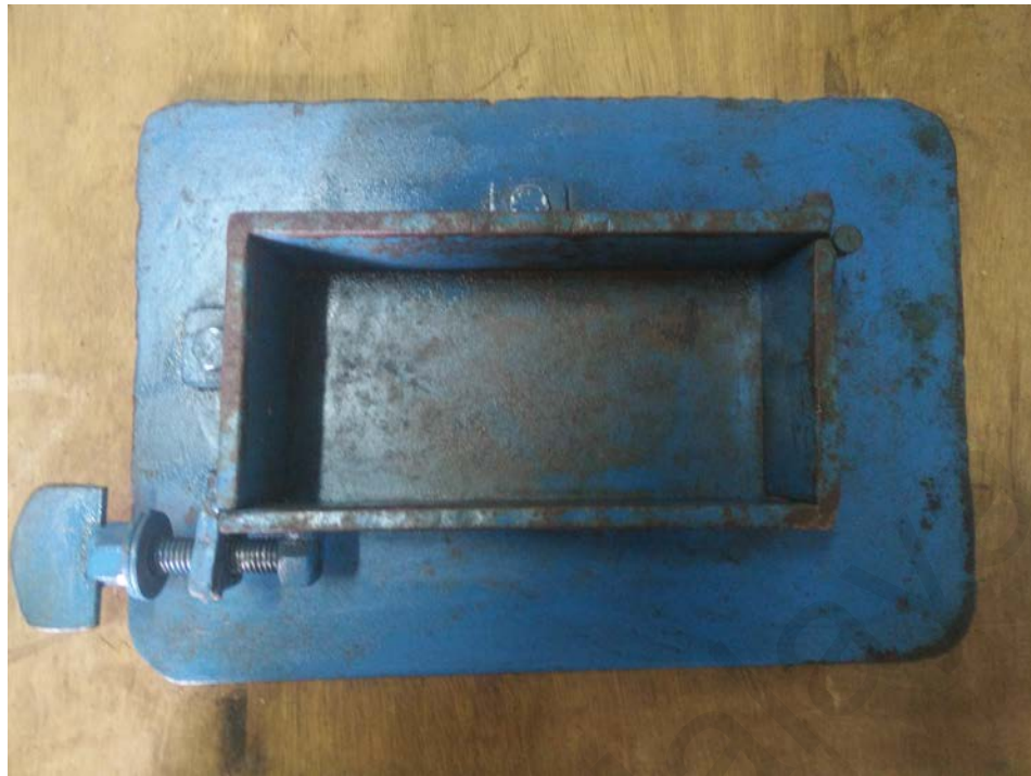
Figure 3.10: Brick mould (10×25×8) cm
