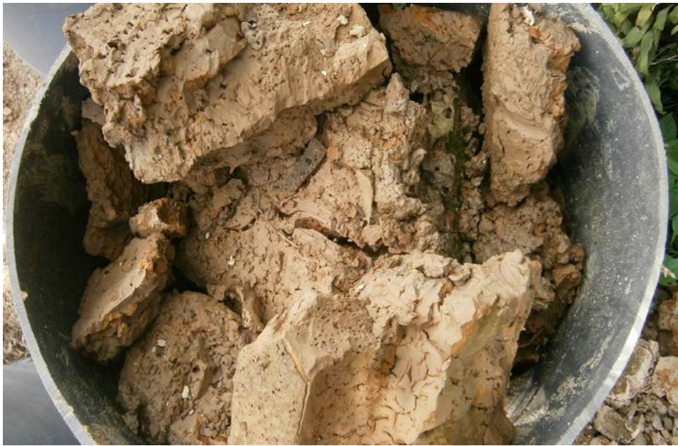
Figure 3.2: Wet sludge collected from drying bed
