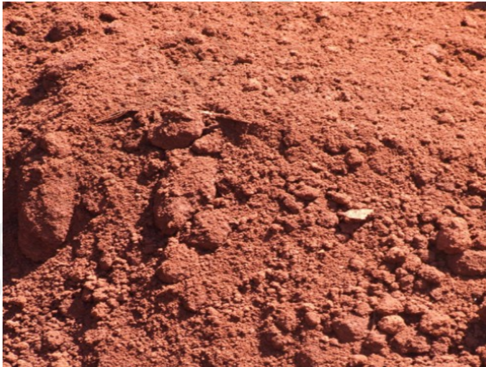
Figure 3.4: Laterite (red earth) taken from local brick manufacturer.
