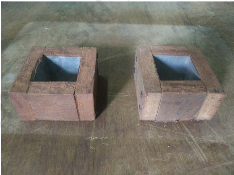
Figure 3.11: Brick mould (5×5×5) cm
