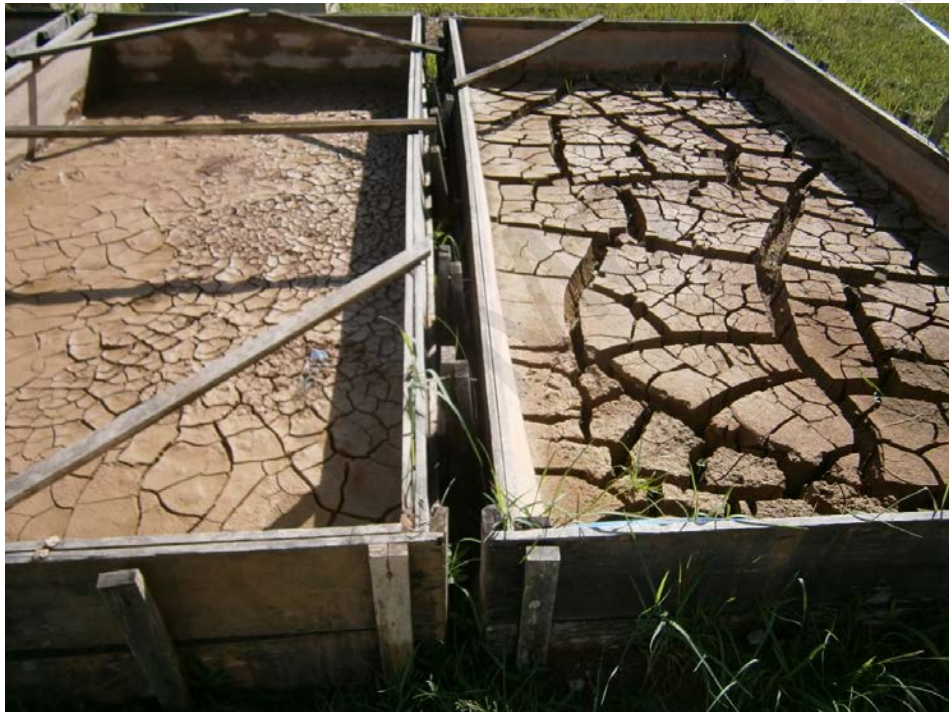
Figure 3.9: WTR obtain from effluent discharge and dried to 50%
