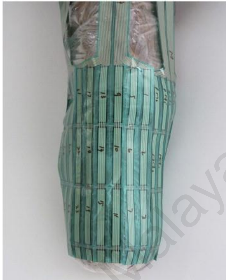
Figure 2.21: Application of piezoelectric transducer to measure interface pressure of the transtibial prosthesis. Reproduced from : (Ali et al., 2012).
