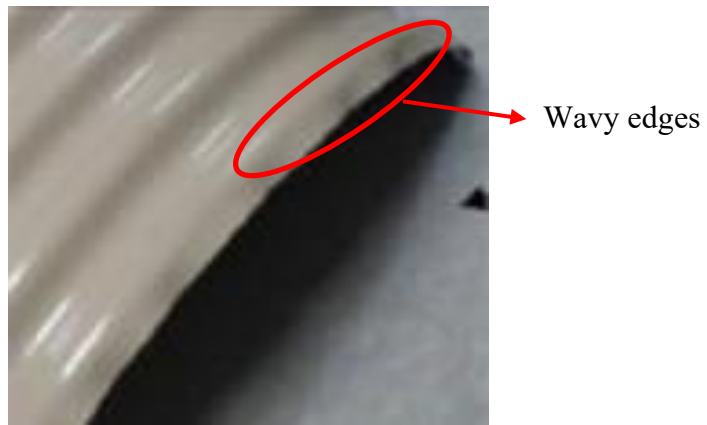
Figure 2.4: Wavy edges in thin-walled sheet (Shim et al., 2017)
