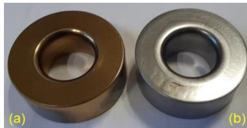
**Figure 3.3 : (a) TiN Coated Die (b) Uncoated Die (Tan CJ et. al 2019)**
