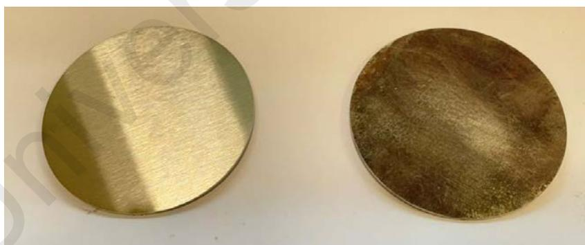
**Figure 4.1 : Non hydrogen charged blanks (left), Hydrogen charged blanks (right)**
