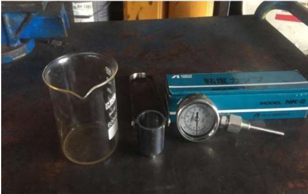
Figure 3.8: Equipment for viscosity cup test
