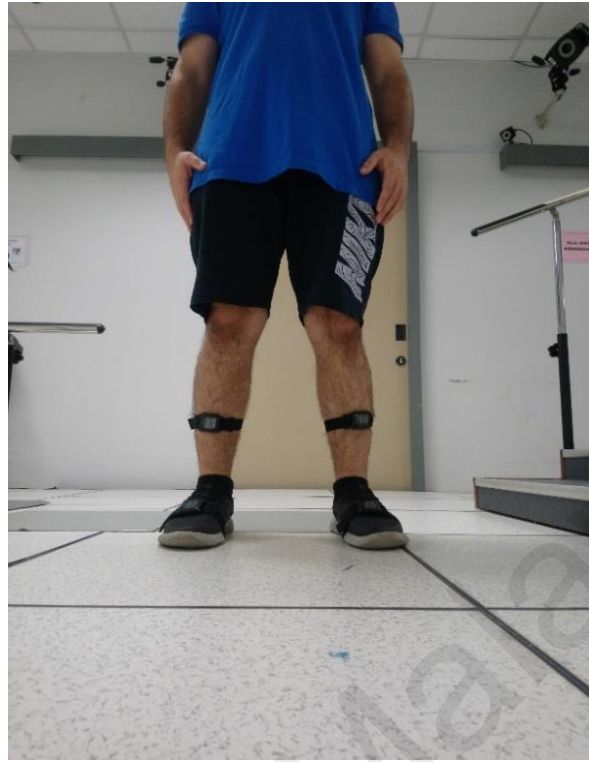
Figure 3.2: A picture of the second subject shows the OPALs sensors placed on the tibia and cuneiform bones in both right and left legs.
